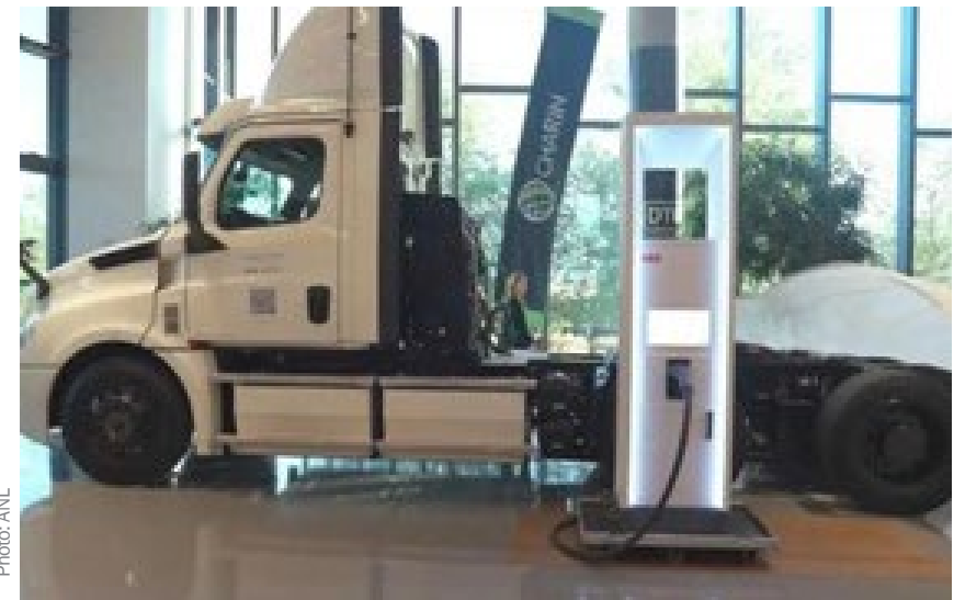
SAE J3271, also called the Megawatt Charging System (MCS), aims to meet the unique high-reliability expectations for commercial vehicles.
