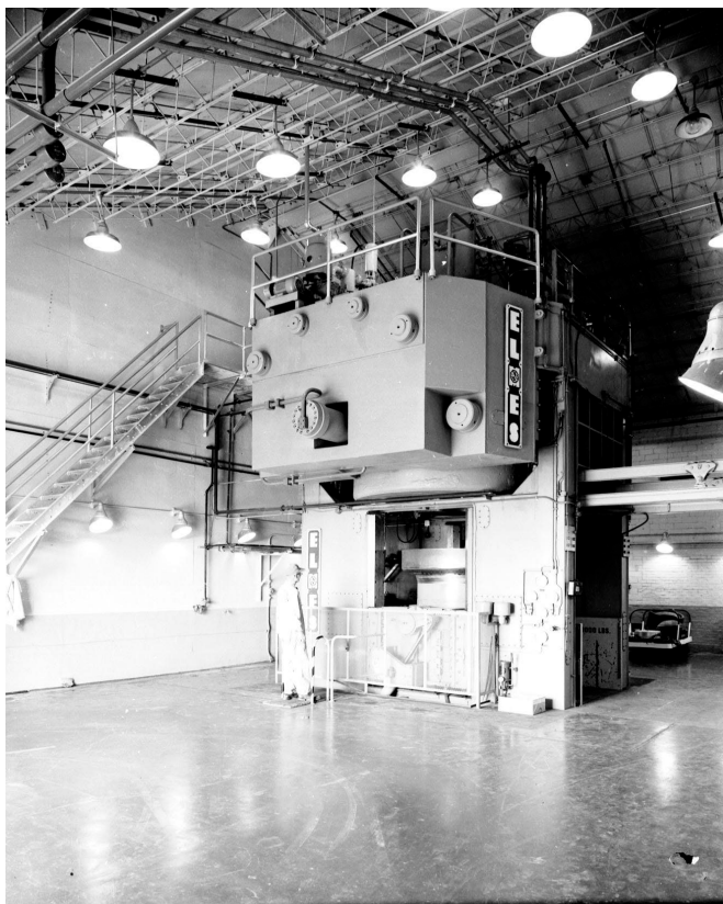
The 20,000psi Elmes Press utilized for high explosives development during the Cold War.
