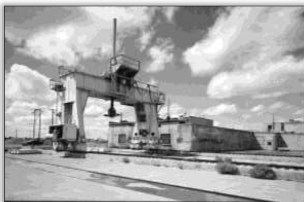
Figure 1: Arco NPG, gantry crane with concussion wall in background, view looking W/SW.
