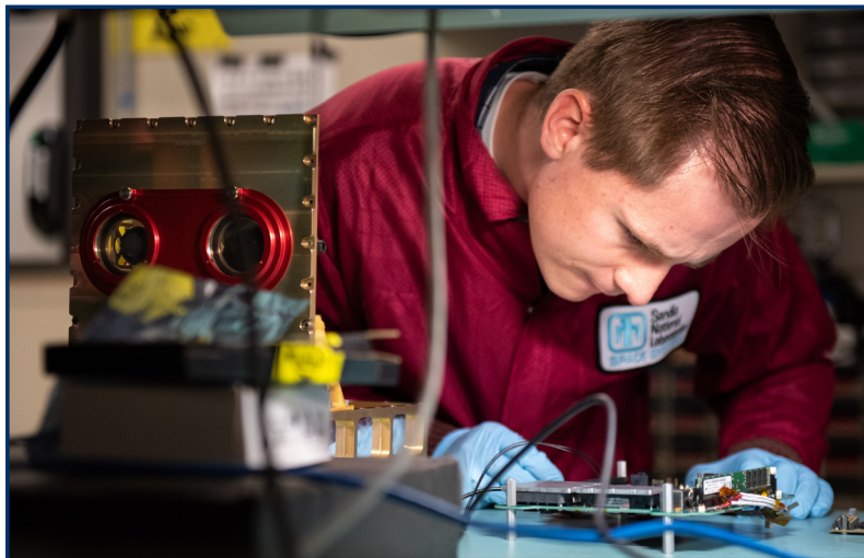
Figure 1: Placing this payload, which includes an advanced microprocessor system on a chip, aboard the International Space Station helps SNL researchers evaluate advanced electronics rapidly for use in national security systems.
