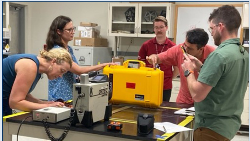
PROACTIVE team members perform a gamma-ray measurement to determine the absence of special nuclear material in a simulated weapons part, as part of a larger verification system exercise at ORNL in August 2023. During the experiment, a building was configured as a mock materials storage facility and outfitted with a variety of sensors including door switches, motion detectors, spectroscopic portal monitors, and cameras. The intent of the experiment was to test and validate a framework for collecting data from a variety of different sensor types, then confirming, storing, and analyzing that data to inform a picture of the facility and identify potential vulnerabilities in the verification process.
