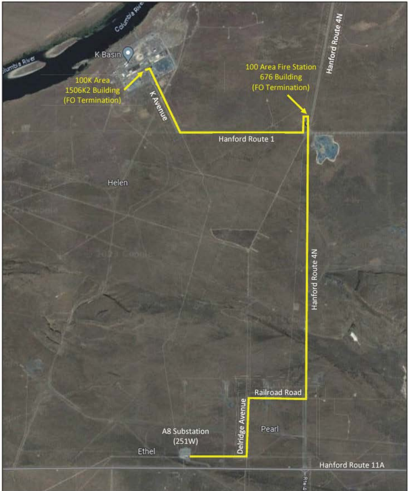
Figure 5 – Aerial Fiber Optic Cable (FO) Route from A8 Substation to 676 and 1506K2 Telecommunications Buildings
