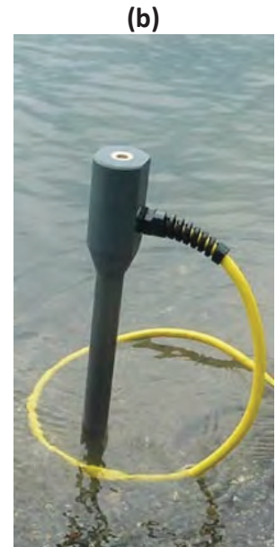
Figure 4. (a) Workflow of the user friendly, Windows-based 1DTempPro code available in the public-domain from USGS for analysis of VTP data to infer specific discharge through a streambed (from Koch et al., 2016); and (b) photograph of TRodX, a commercially available VTP probe ( https://nevada.usgs.gov/TROD/measurements.html ) .
