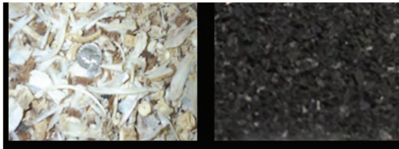
Figure 2. Two key exemplars of Bio-Apatite media – Apatite II (left) and Bone char (right).
