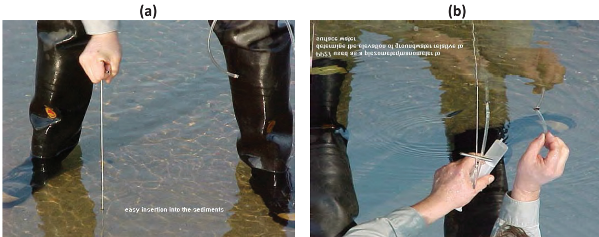
Figure 2. (a) Installation of a MHE PushPoint Sampler, and (b) sampling using a syringe pump. http://www.mheproducts.com/insertion.jpg .
