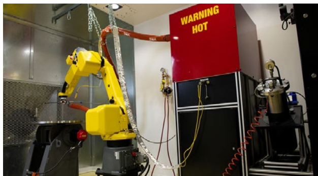
Pacific Northwest National Laboratory is working on a new spray coating to repair dam turbines. Photo from Andrea Starr, Pacific Northwest National Laboratory
