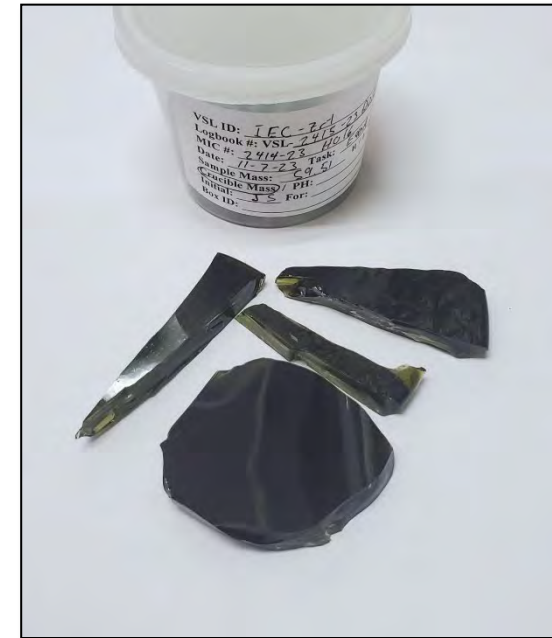
Glass made with Zr-calcine at 35% waste loading
