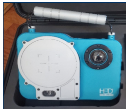
Commercial gamma-ray imagers from H3D based on room-temperature detectors are a recent innovation enabling this work. Photo credit: Klaus-Peter Ziock, ORNL.
