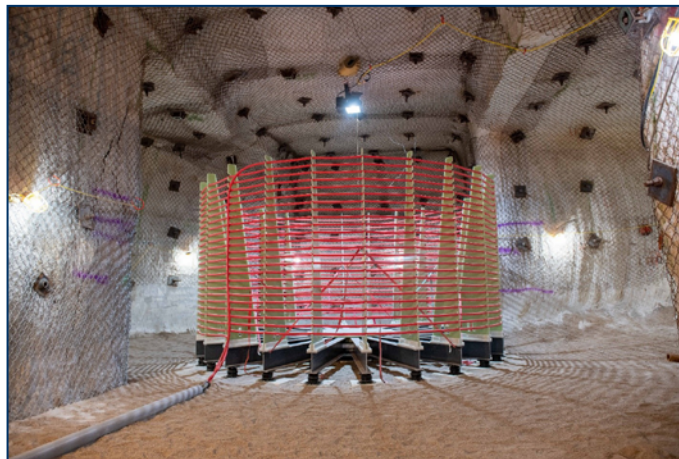
The equipment in P-Tunnel used to generate the synthetic electromagnetic signal used in the April 2022 PE1 experiment.
