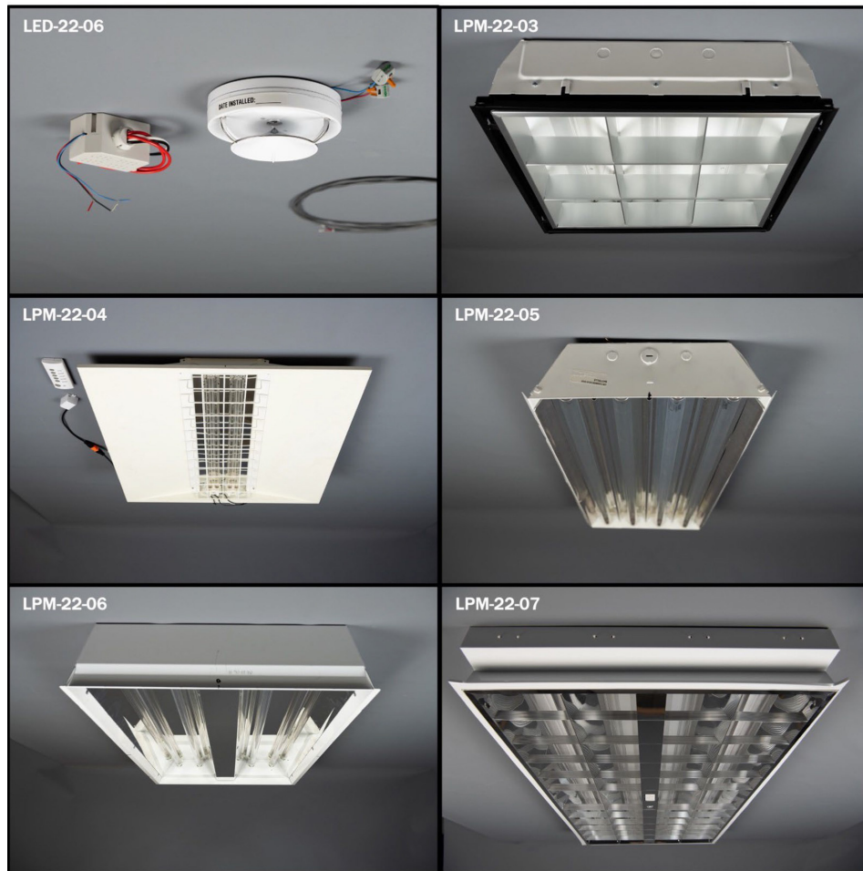
Figure 2. LED and LPM whole-room luminaires, viewed from below and to one side. LED-22-06 had a 5-in. diameter and protruded 2.1 in. below ceiling. LPM-22-03 and LPM-22-04 were 2-ft by 2-ft troffers, measuring 2 ft on each side in plan. LPM-22-05 was a high-bay luminaire measuring 14-in. by 48-in. in plan. LPM-22-06 and LPM-22-07 were 2-ft by 2-ft troffers. Troffers are intended to be recessed into the ceiling, but are shown surface mounted.
