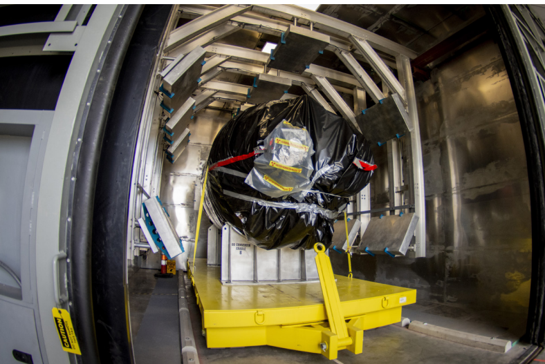
Process gas equipment is scanned in LINAS chamber as technicians finalize methods for measuring deposits from past operations.
