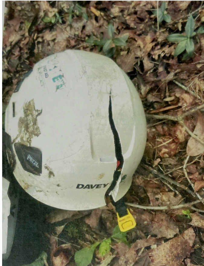
Figure 3-2. Split to Helmet after the Dead Limb Piece Made Contact (photo taken by ORPD)
