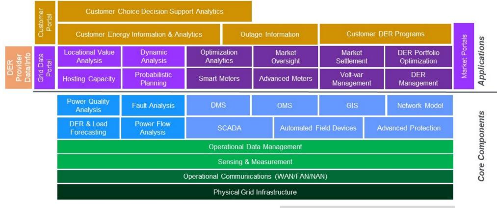
Green - Core Cyber-physical layer Blue - Core Planning & Operational systems Purple - Applications for Planning, Grid & Market Operations Gold - Applications for Customer Engagement with Grid Technologies Orange - DER Provider Application
