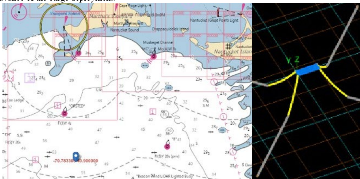
Figure 5. Nautical chart of the location of the Barge (right) 4-point mooring design of the Barge.
