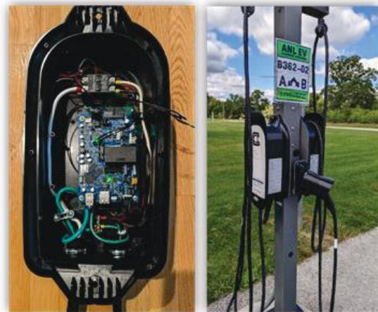
Figure II.4.3.13 Left: Argonne SpEC II module integrated into HCS-40P enclosure. Right: Two proof of concept OptiQ EVSE deployed for Argonne employee use at Argonne.
