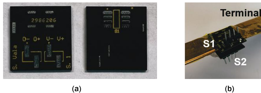
Figure I.1.23.9 (a) Designed PCB for the GMR current sensors, (b) TGS method implementation on AC copper terminal.
