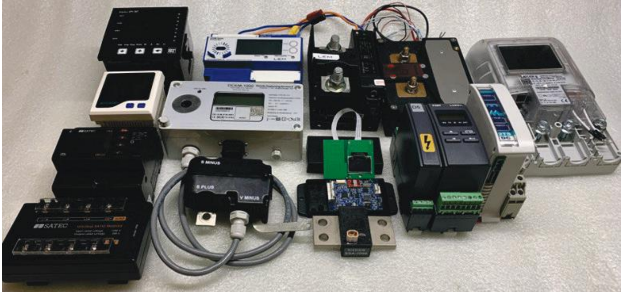
Figure II.6.7.2 Ten meter and current sensor benchmark test articles. (clockwise, top left); Rish, LEM, Tritium, Isabellenhuette, MeasurLogic, Lumel, EVOKE, Porsche Engineering Services, Satec, and AccuEnergy (Source: ANL).
