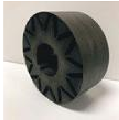
Figure I.1.16.4 Fabricated HF-10 rotor lamination
