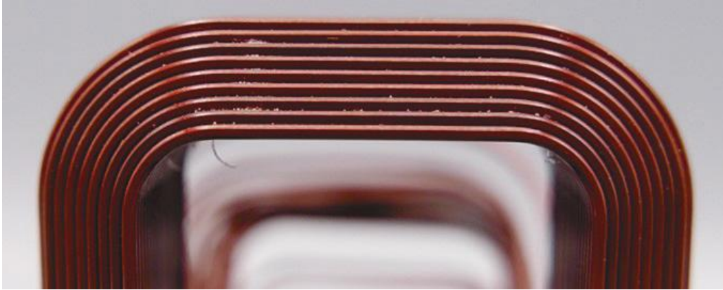
Figure I.1.22.3 Representative example of a die compressed coil using a spaced orthocyclic winding without dislocations or over deformed wires.
