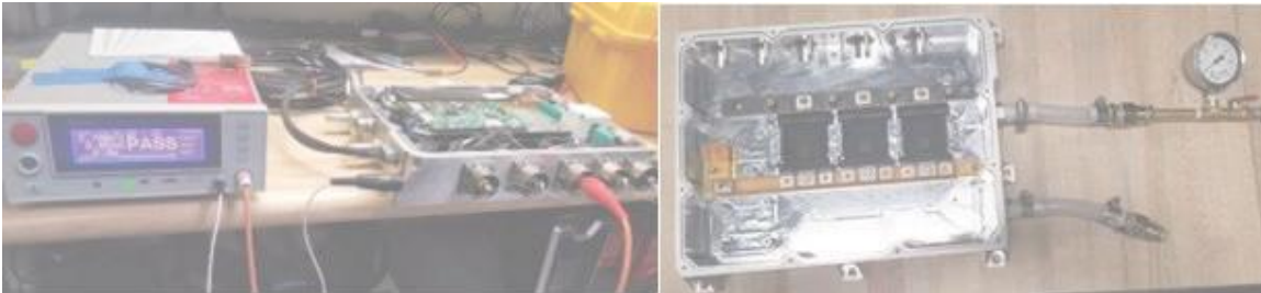
Figure II.1.4.3 HiPot and Leak Tests
