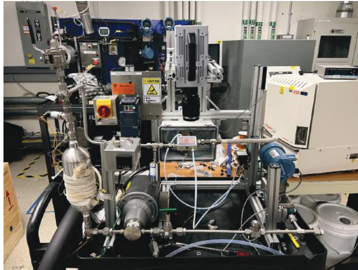
Figure I.1.15.5 Completed flow loop
