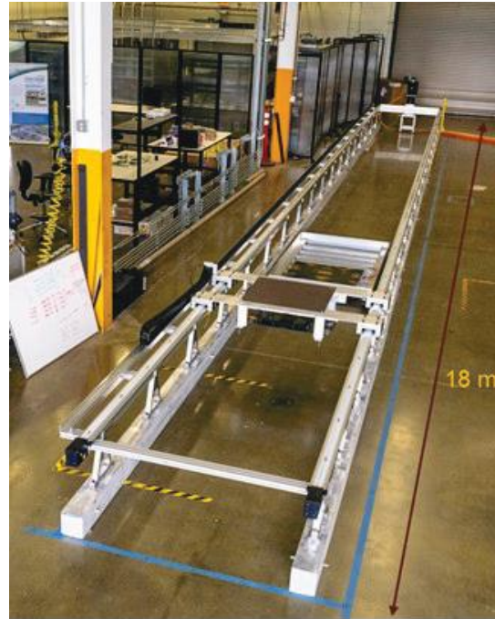
Figure II.3.1.4 Top view of the ORNL DICE depicting the overall track length of 18 m.
