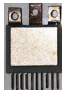
Figure I.1.24.4 A fabricated double-side cooled SiC phase-leg power module encapsulated by EP-2000 for 200°C-T j operation.
