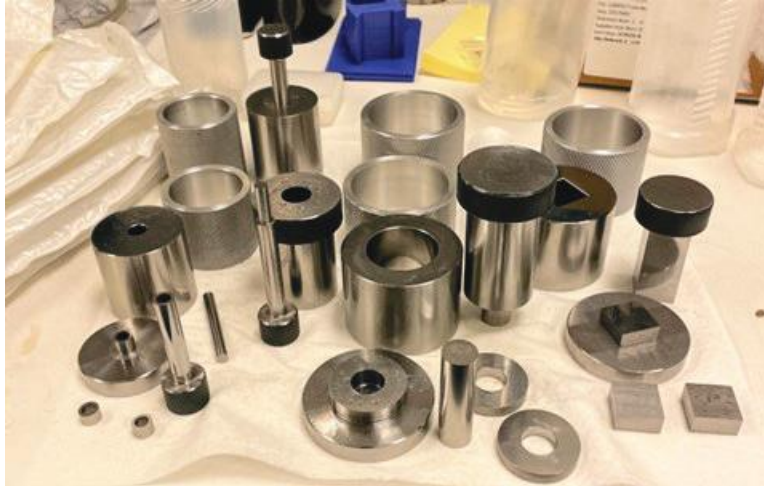
Figure I.1.14.7 New die for pressing larger toroids and cubes.
