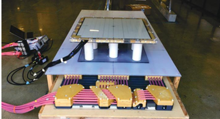
Figure II.3.1.2 Laboratory setup for characterization of 200 kW DWPT system prior to concretizing the ground coil.
