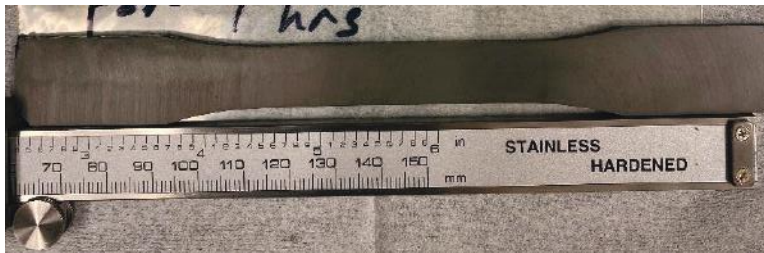
Figure I.1.14.3 Dog bone structure ready for measurement at NREL.
