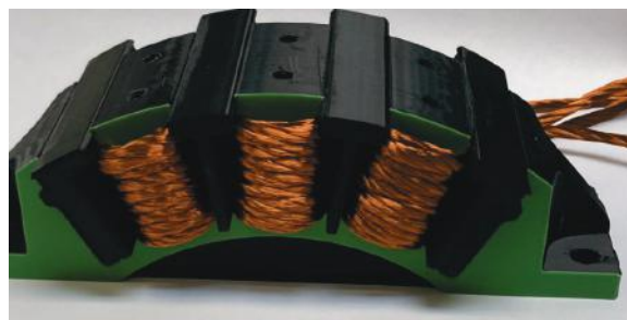
Figure I.1.3.2 Winding trials on a 3D-printed stator.
