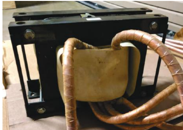
Figure II.2.3.16: 175 kVA 1000V, 800 V Transformer based on Nanocrystalline core and Litz wire.
