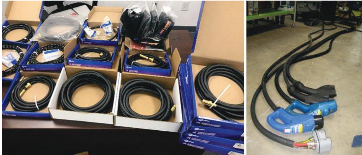
Figure II.6.7.3. Liquid cooled and conventional CCS-CHAdeMO charging cables evaluated in benchmark study (Source: ANL).
