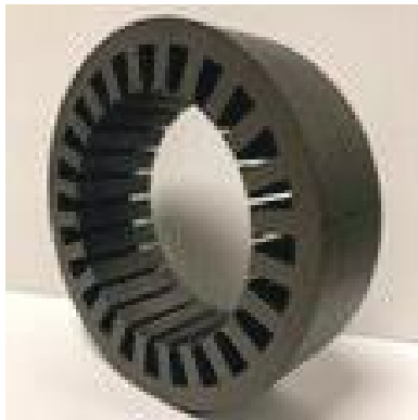
Figure I.1.16.3 Fabricated HF-10 stator lamination
