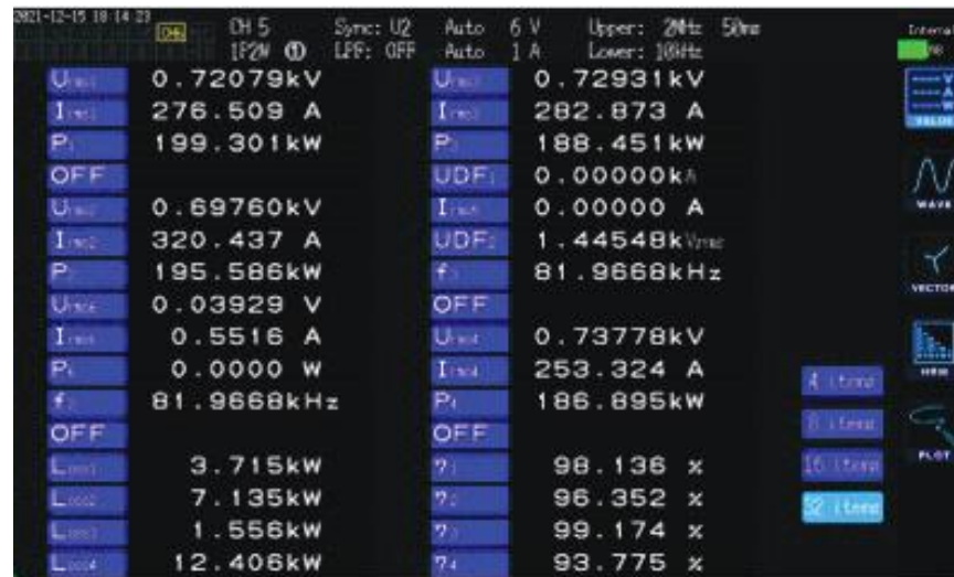
Figure II.3.1.7 Power transfer validation of 200 kW DWPT couplers with the transmitter embedded in 500 PSI epoxy grout. The output power was 186.8 kW, and efficiency was 93.775%.
