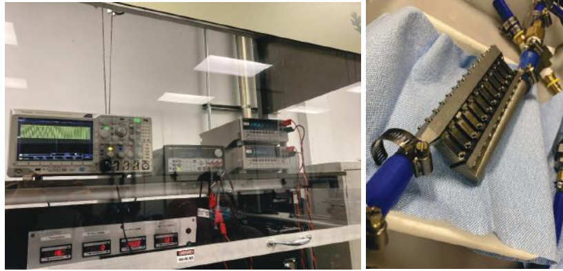
Figure I.1.2.4 Photos of cooling subsystem pressure test setup.
