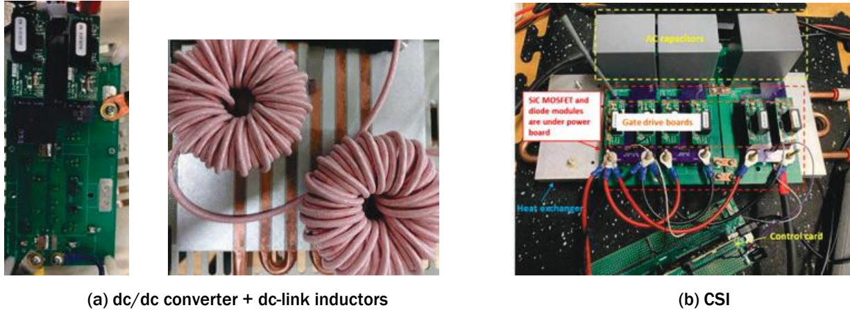
Figure I.1.18.2 Fabricated benchtop prototype CSI + dc/dc converter system.
