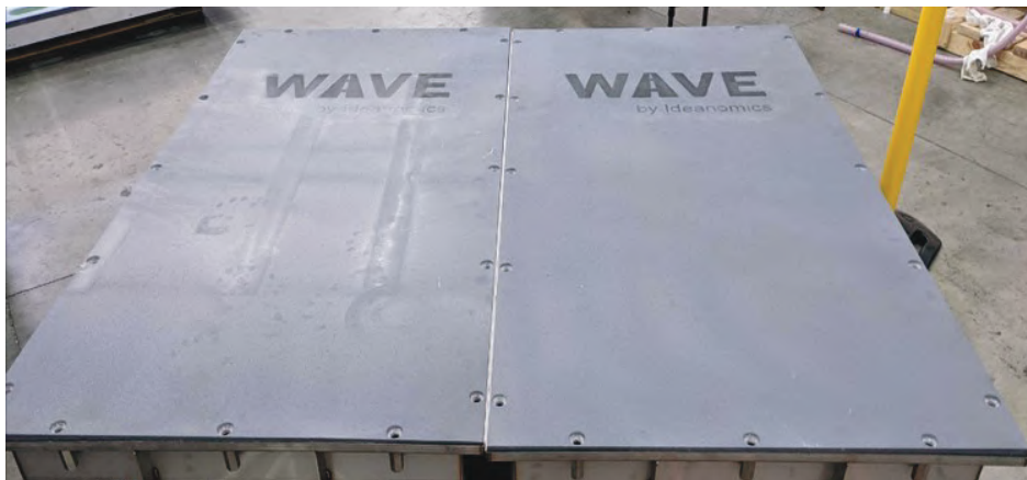
Figure II.1.8.4 Primary Charging Pads
