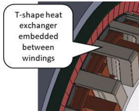
Figure I.1.7.4. T-shape heat exchangers embedded between stator windings. Illustration by Bidzina Kekelia, NREL
