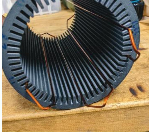
Figure I.1.22.5 Partial continuous shaped conductor continuous wave winding inserted into a mockup 3D printed stator.
