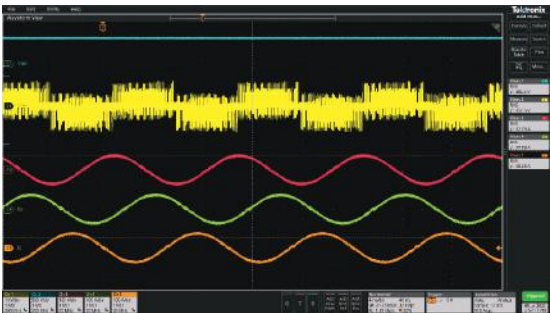
Figure I.1.2.8 Operating waveforms. From top to bottom: DC bus voltage, line-to-line voltage, and three-phase currents.
