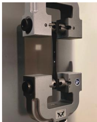
Figure I.1.10.1 Mechanical tensile test setup with sample loaded prior to testing. Photo by Emily Cousineau, NREL
