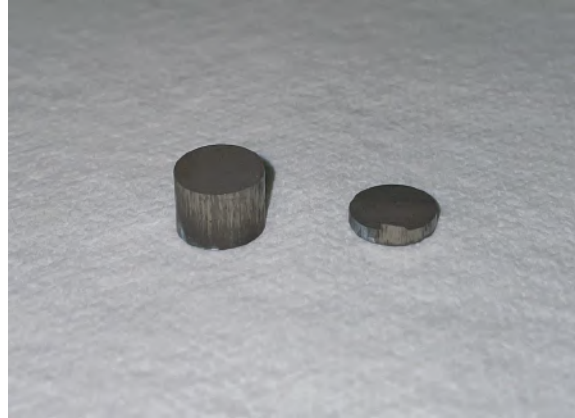
Figure I.1.14.5 75.3 vol.% Fe 4 N in epoxy SMC. The shorter cylinder was cut using a diamond saw for VSM analysis.
