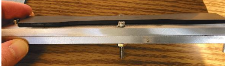
Figure I.1.14.2 Jig to prevent bowing of dog bone structures during final cure with a completed test structure resting on top.
