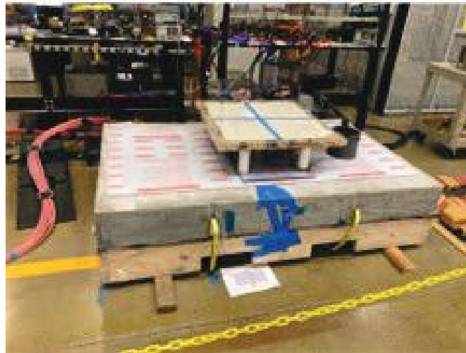
Figure II.3.3.5. Concretized 200 kW transmitter setup for electrical characterization.
