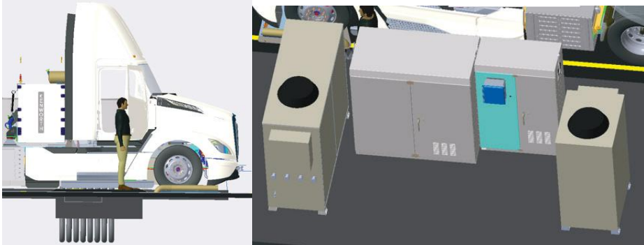
Figure II.1.1.3 Portland, Seattle facility drawings of electronics cabinet layout showing available space to adequately house the utility equipment, charger electronics and charge pad and allow adequate clearance for unobstructed tractor trailer operations around the equipment.
