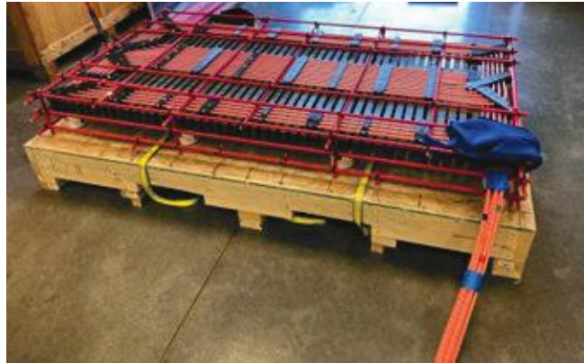
Figure II.3.3.2. The 200 kW DWPT transmitter.
