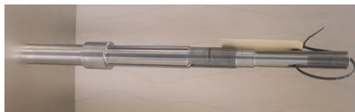
Figure I.2.8.4 Designed and prototyped shaft of the motor
