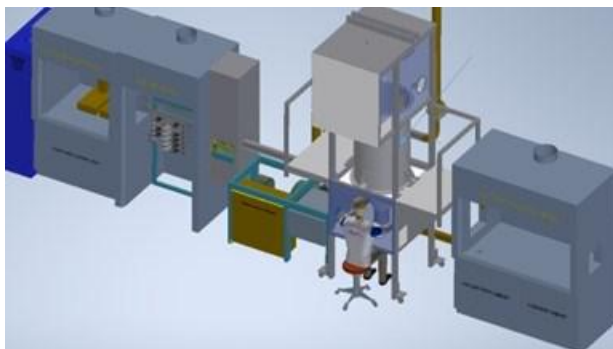
Figure II.2.4 FSP configuration for 500 g/hour production
