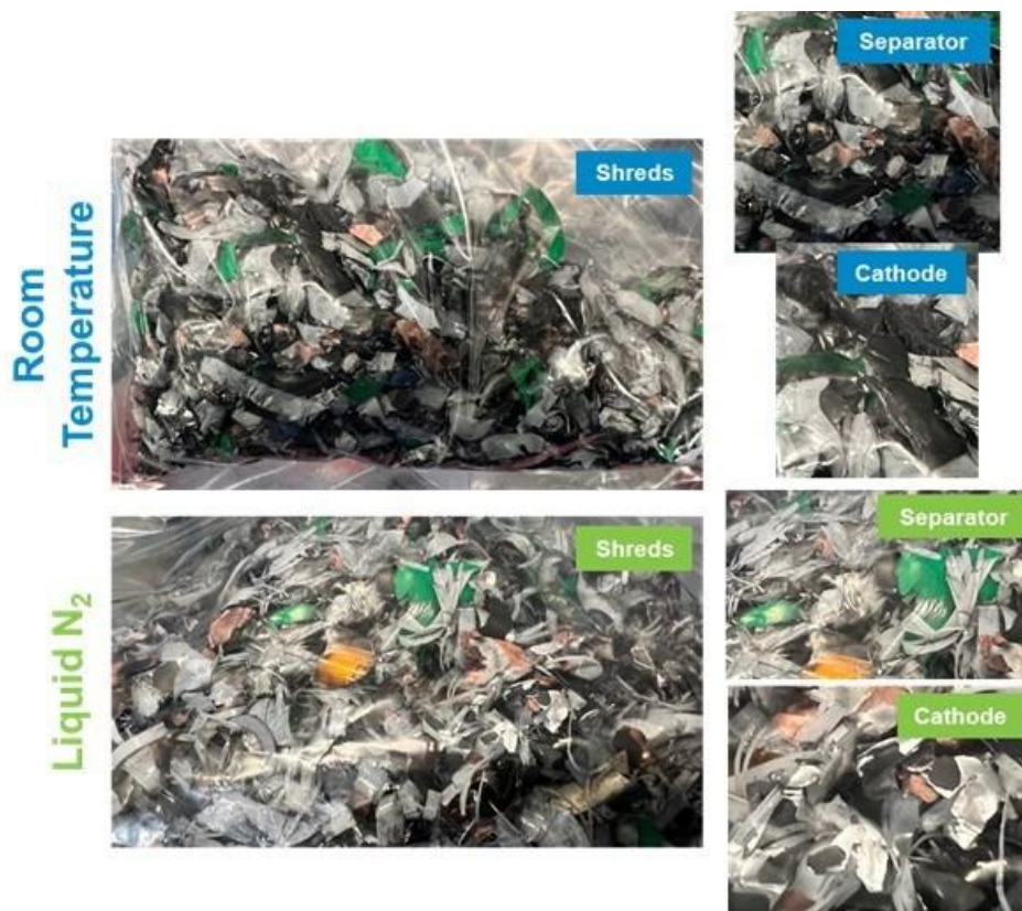
Figure III.3.62 Shredding cycled 18650 cylindrical cells under inert atmosphere at room temperature (top) and after freezing in liquid nitrogen (bottom)
