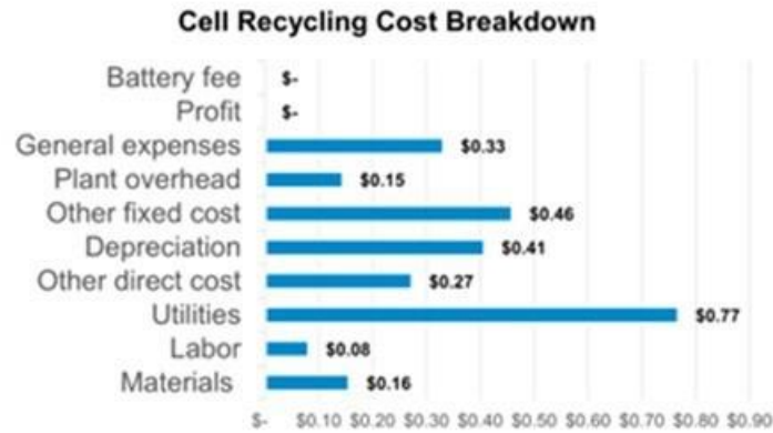
Figure III.3.77 EverBatt cost analysis of the recycling of graphite into graphene from graphite on copper foil. Cost is in $/kg of graphite recycled.
