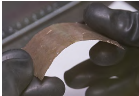
Figure XVI.7.9 Ternary glass separator with 0.75 mS/cm ionic conductivity and 110 μm thickness.
