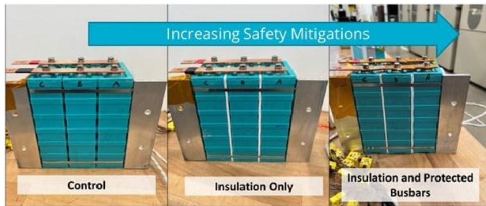
Figure V.1.10 Three different thermal control strategies were used for three 20 Ahr lithium iron phosphate cells connected in parallel.
