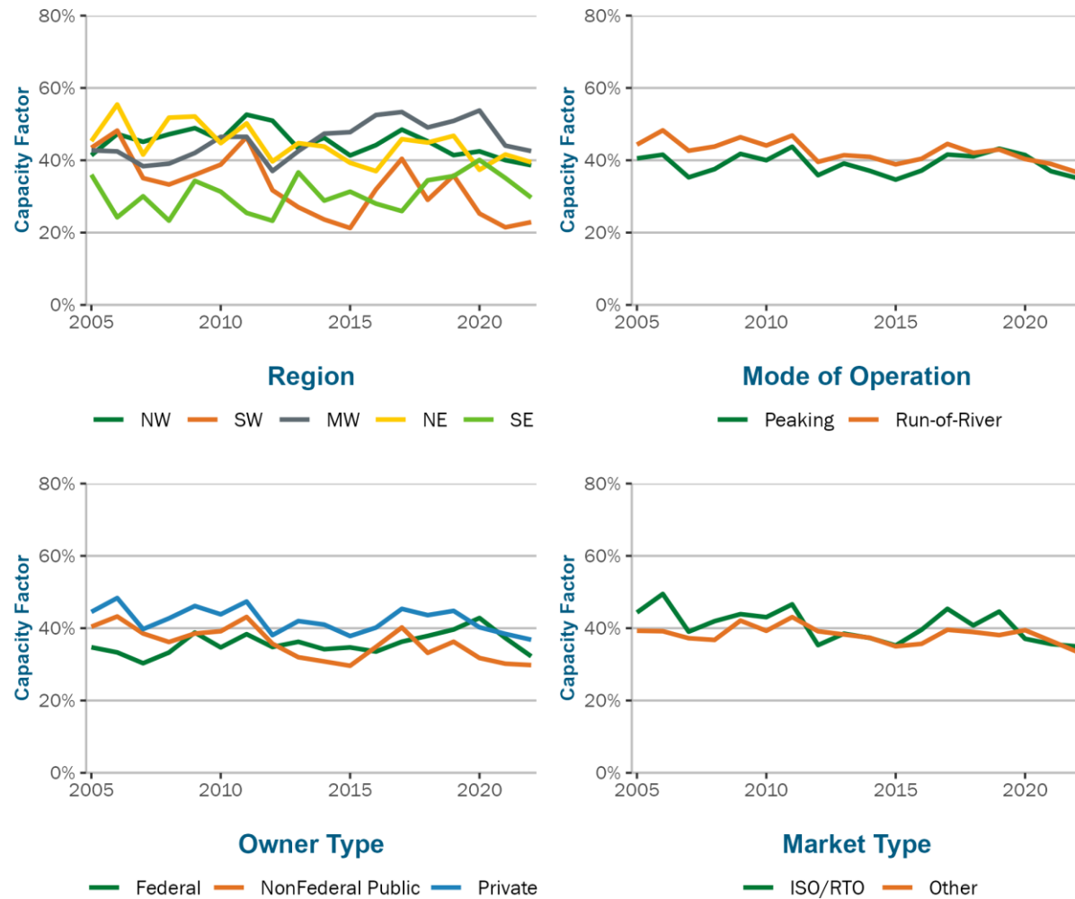
Annual average hydropower capacity factor by region, mode of operation, owner type, and market type
