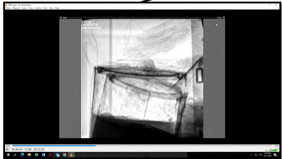
High Energy Real Time Radiography Scan of a Sealed Container
