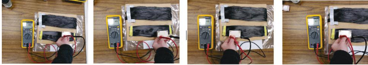
Figure II.3.1.3. Random resistance measurements of the continuous batch sample. Most of the values are in the 1\Omega range or below, as shown in the pictures. This value is typical of fiber that has been processed at 1200^\circ\text{C} or higher. (Note: the unknown number of filaments between the probes is a limitation of the accuracy of this method.) Source: ORNL.
