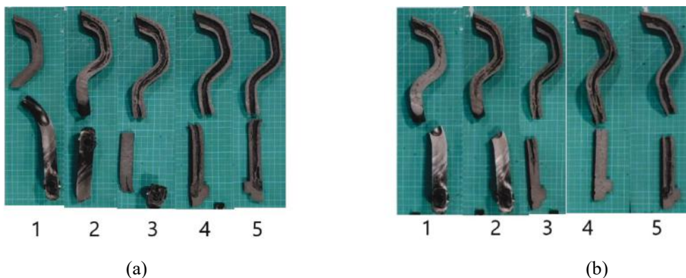
Figure II.3.1.141. Progression of hot runner degree of hollow after water-assist is turned on. (a) A seven-second pack sample. (b) A ten-second pack sample. Source: Ford Motor Company.
