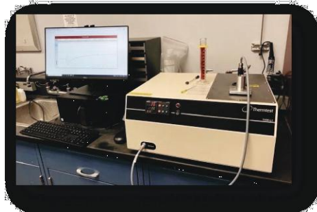
Figure I.1.2.16. The addition of 0.5% CNTs increased the thermal conductivity of PAO and PAG base oils by 7%–8% and 8%–10%, respectively. Source: ORNL.
