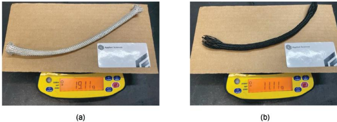
Figure II.3.2.21. Weight comparison between two braided harnesses: (a) traditional copper plated metal harness and (b) 40% lighter PVC/CNF composite fabricated by ASI. Source: ASI.
