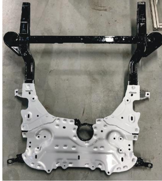
Figure II.4.2.6. Final prototype component with Al painted gray and steel black. Source: The Ohio State University.
