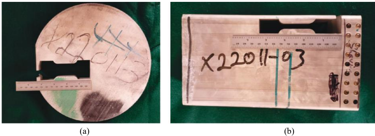
Figure II.2.2.5. (a) Remnants from cast billet. (b) Section from an extrusion. Source: ORNL.
