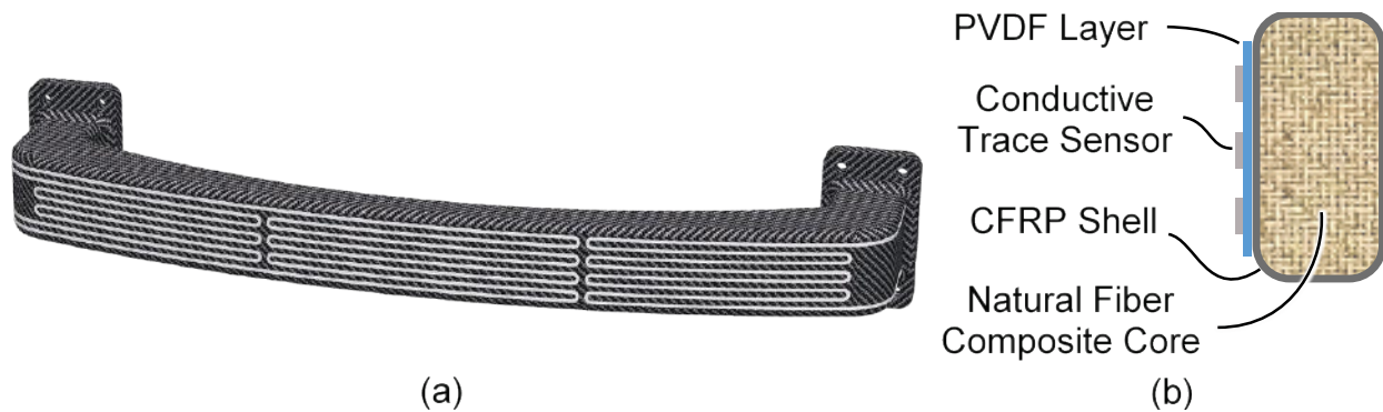
Figure II.3.2.1. (a) SLIC bumper beam. (b) Cross section schematic of SLIC bumper beam.
