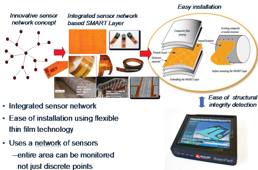
Figure II.3.2.6. SMART layer sensors. Source: Acellent Technologies, Inc.
