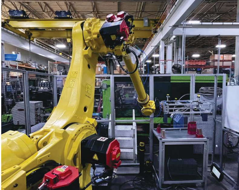
Figure II.3.1.152. The pick-and-place robot automation cell. Source: Ford Motor Company.
