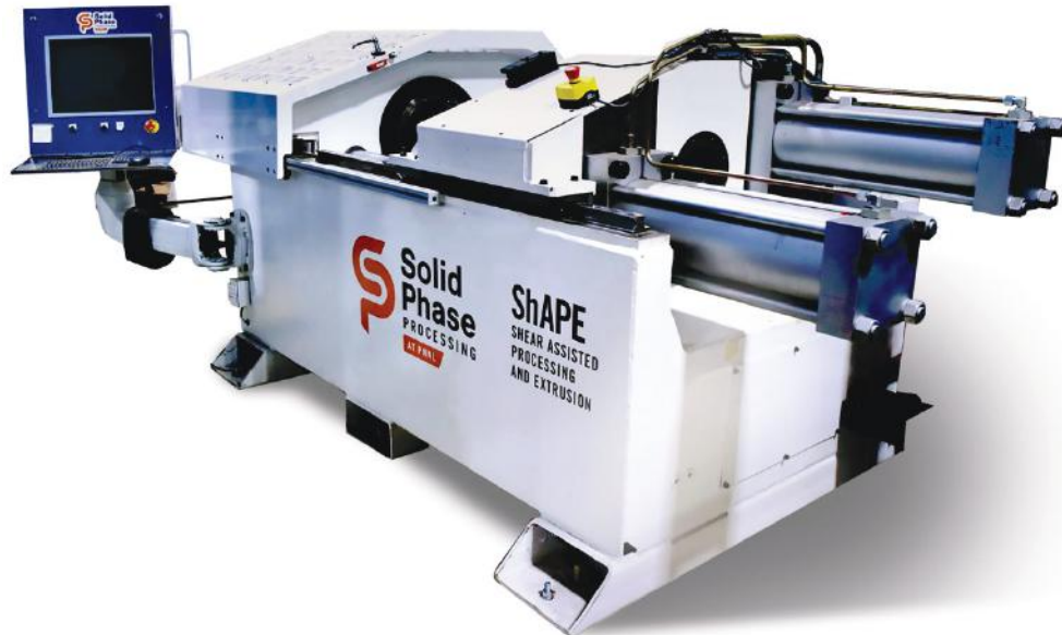
Figure II.2.1.1. ShAPE machine installed in PNNL's Solid-Phase Processing Laboratory. Source: PNNL.
