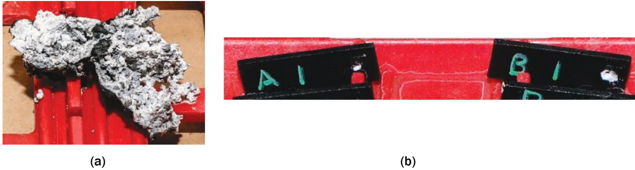
Figure II.2.2.4. Visual evaluation of corrosion tested coupons: (a) AM60B control and (b) Alloy #1. Source: FCA US LLC.
