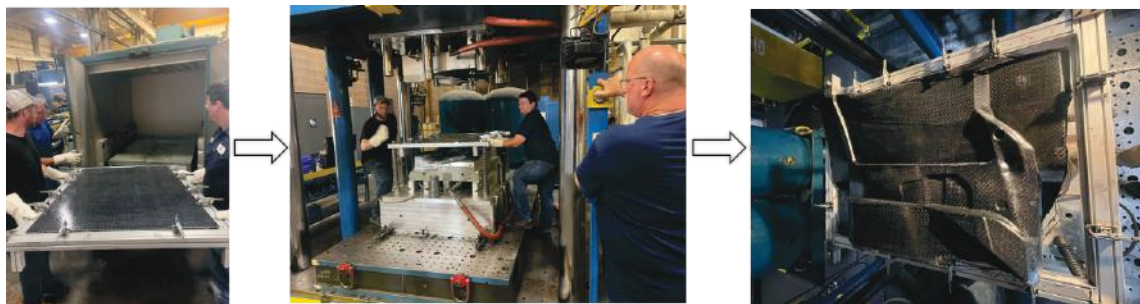
Figure II.3.1.129. Process flow for stamping: heating, transport and forming of material. Source: Clemson University.
