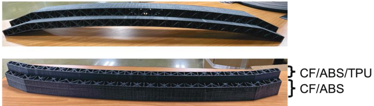
Figure II.3.1.16. Full-scale multimaterial lattice-based bumper. Source: ORNL.
