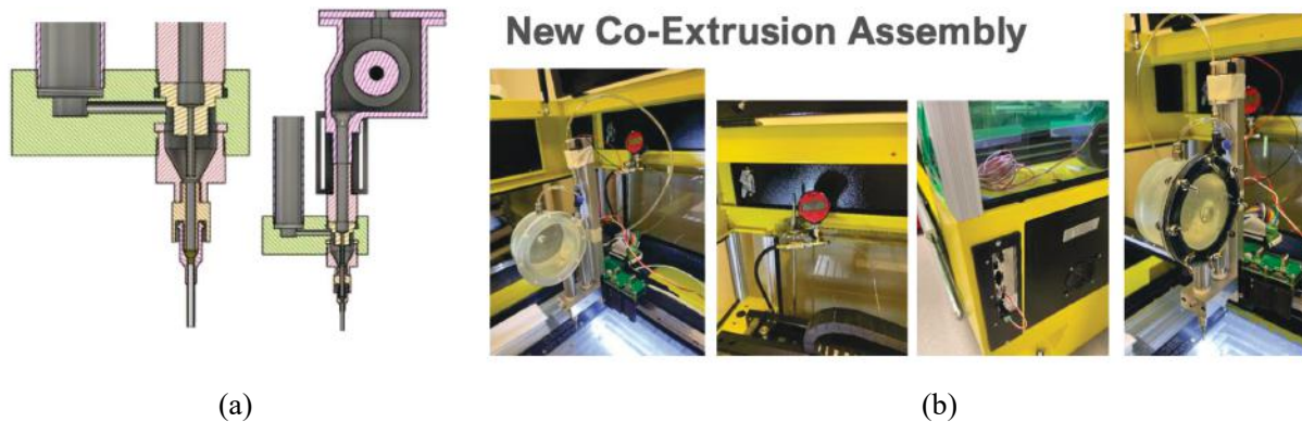
Figure II.3.1.27. (a) 3D-printing of epoxy and continuous CF was initially achieved with the modified Hyrel attachment; however, results were not ideal and backpressure flows are still a problem. (b) A new co-extrusion assembly was designed to have both the fiber and epoxy matrix under the same pressure environment. Source: ORNL.
