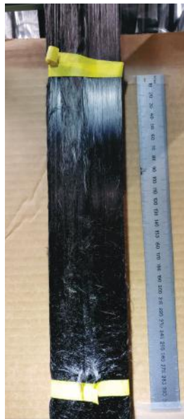
Figure II.3.1.2. Picture of a continuous sample of 300k filaments ribbon coming out of the HTC before the split. The yellow tags delimit the processing conditions. Minor damage can be noticed in the center left of the sample. Source: ORNL.
