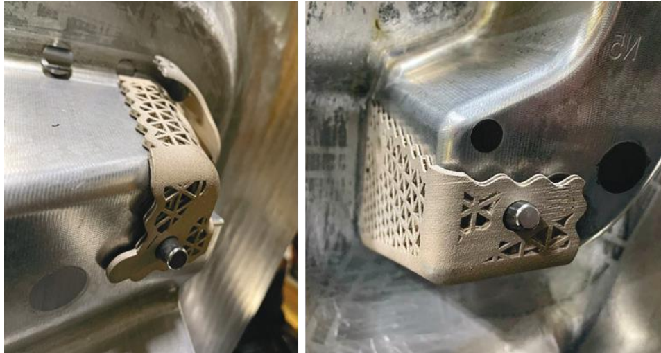
Figure II.3.1.148. Close-up of inserts placed in the molding tool. Source: Ford Motor Company.
