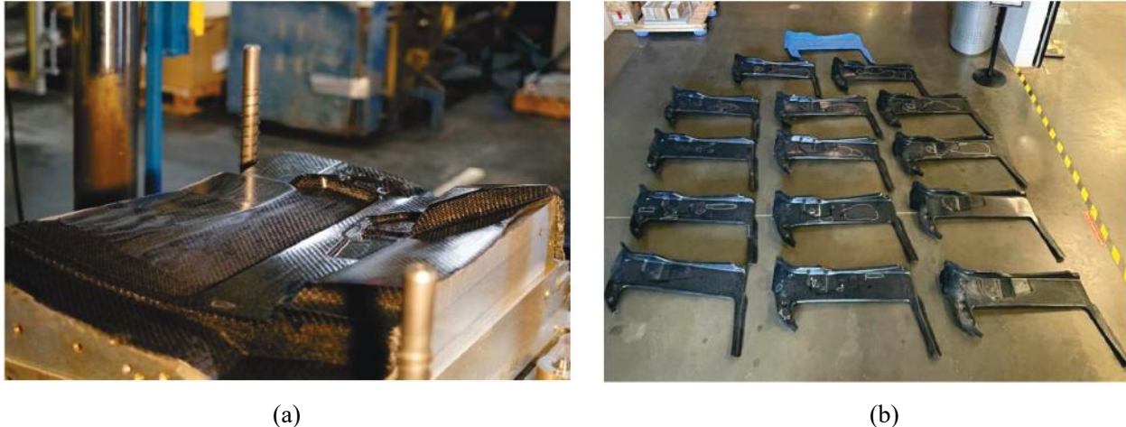
Figure II.3.1.131. (a) Formed inner beltline part on the heated tool. (b) Post-processed parts being evaluated. Source: Clemson University.
