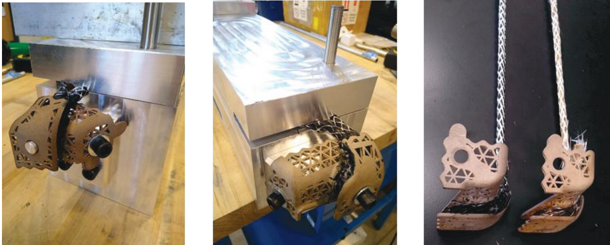
Figure II.3.1.143. M-TOW preforms produced in support of injection overmolding studies. Source: Ford Motor Company.
