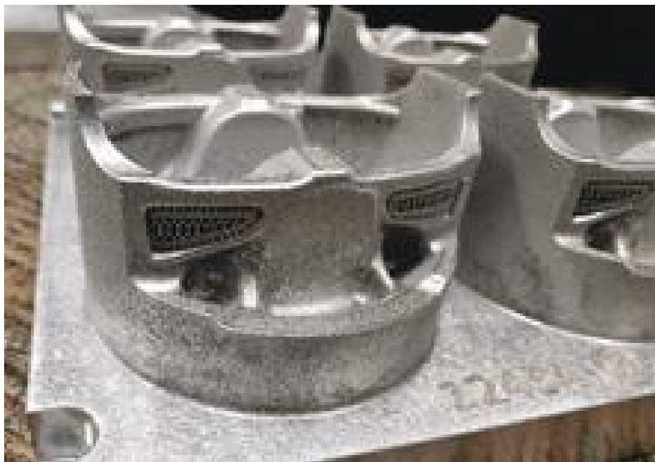
Figure I.2.2.8. AM printed PHASE 2 pistons. Source: ORNL.
