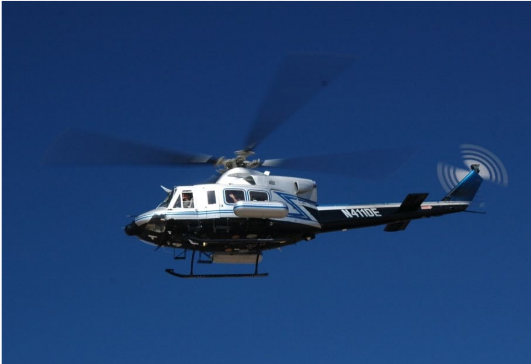
Figure 2. RLS Bell 412 Helicopter with Externally Mounted AMS Detector Pods
