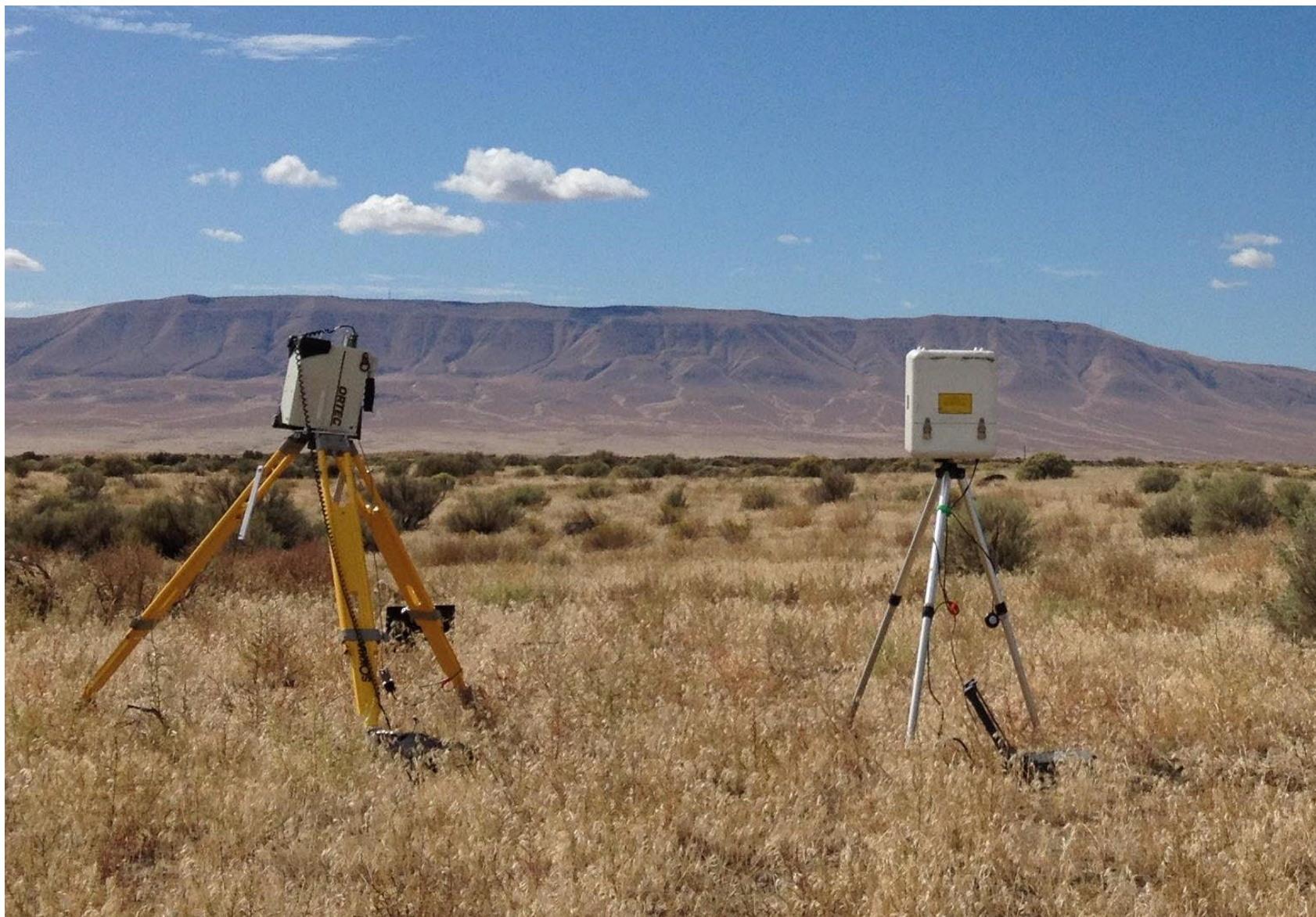
Figure 6. Ground Truth Measurements with HPGe Detector and Pressurized Ion Chamber
