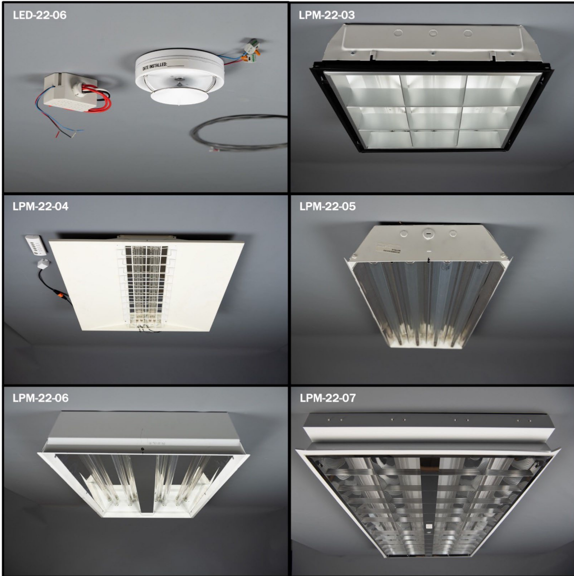
Figure 2. LED and LPM whole-room luminaires, viewed from below and to one side. LED-22-06 had a 5-inch diameter and protruded 2.1 inches below ceiling. LPM-22-03 and LPM-22-04 were 2x2 troffers, measuring 2 feet on each side in plan. LPM-22-05 was a high-bay luminaire measuring 14x48 inches in plan. LPM-22-06 and LPM-22-07 were 2x4 troffers. Troffers are intended to be recessed into the ceiling but are shown surface-mounted. Photo credit: PNNL (Andrea Starr).
