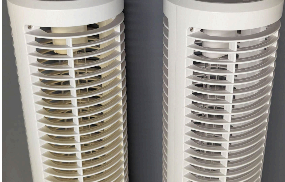
Figure 7. LPM-22-02C after three days of gonio testing (left) and unused LPM-22-02B (right).
