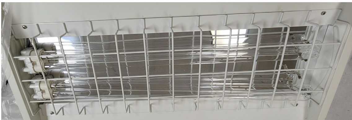
Figure 31. Close-up view of LPM-22-04A. One of the two lamps in the unit received was still attached to its socket (at lower left) but had popped out of its support clip (at lower right).
