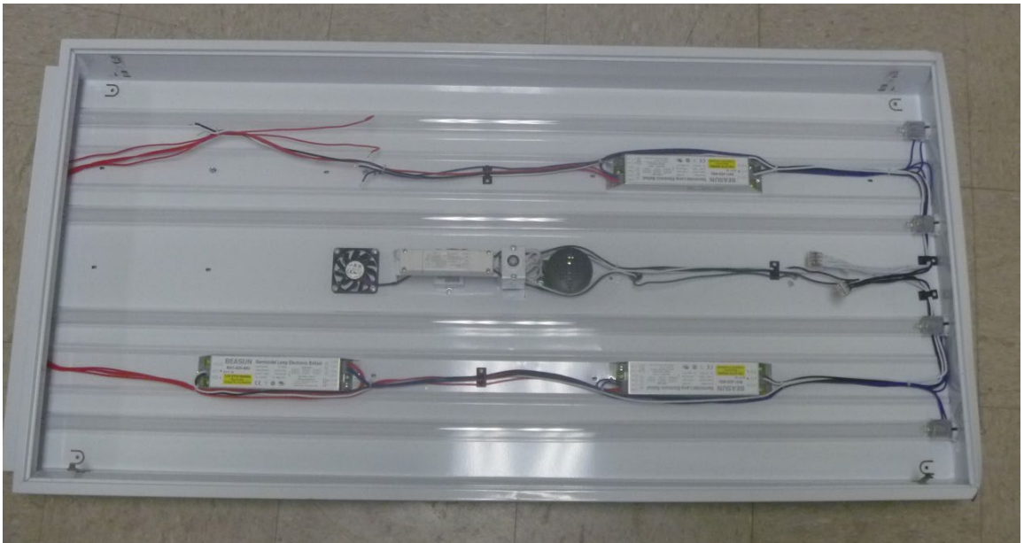
Figure 32. Two views of LPM-22-07A. Image (a) shows damage to corners of housings typical of all units received. Image (b) shows the internal ballast compartment, where one of the four 1-lamp ballasts was missing. Notably, the internal fan for this product is visible left of center.
