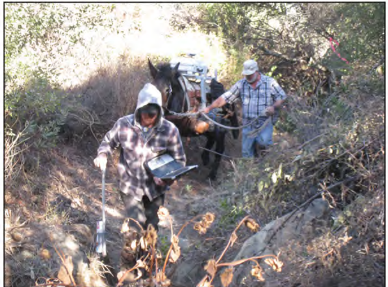
Photo 1D - Gamma scanning in a riparian zone by MMGS.
