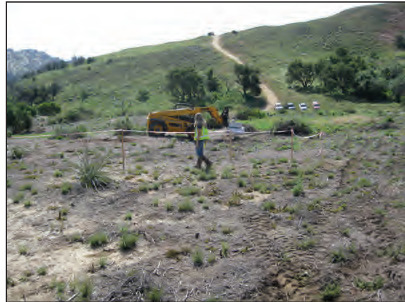
Plate 3D – ERGS gamma scanning in Subarea 8 South (SS-49), with a Branton's milkvetch patch marked as restricted adjacent to ERGS. May 5, 2011.
