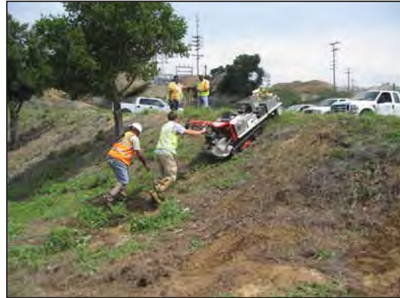
Plate 1B - Modified Canycom track-mounted gamma scanner being operated in Subarea 6 (SS-35).
