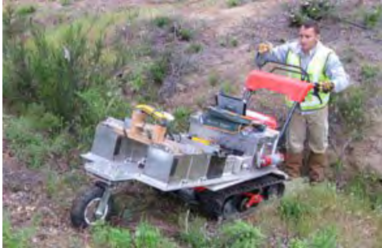
Figure 6 Dual Detector Track Mounted Gamma Scanner Detection System
