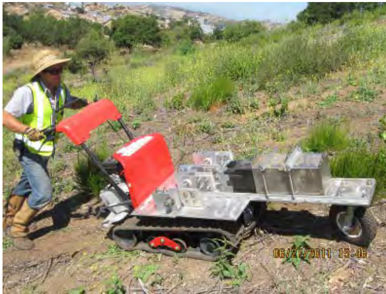
Figure 7 Single Detector Track Mounted Gamma Scanner Detection System
