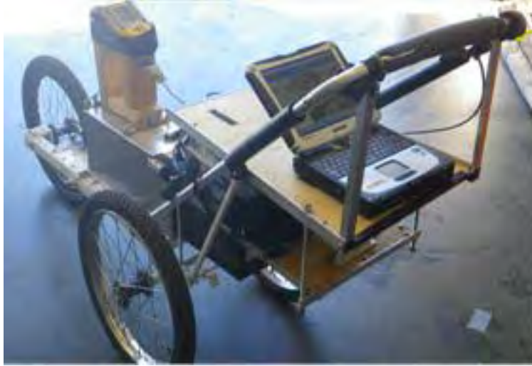
Figure 8 Wheel Mounted Gamma Scanner Detection System
