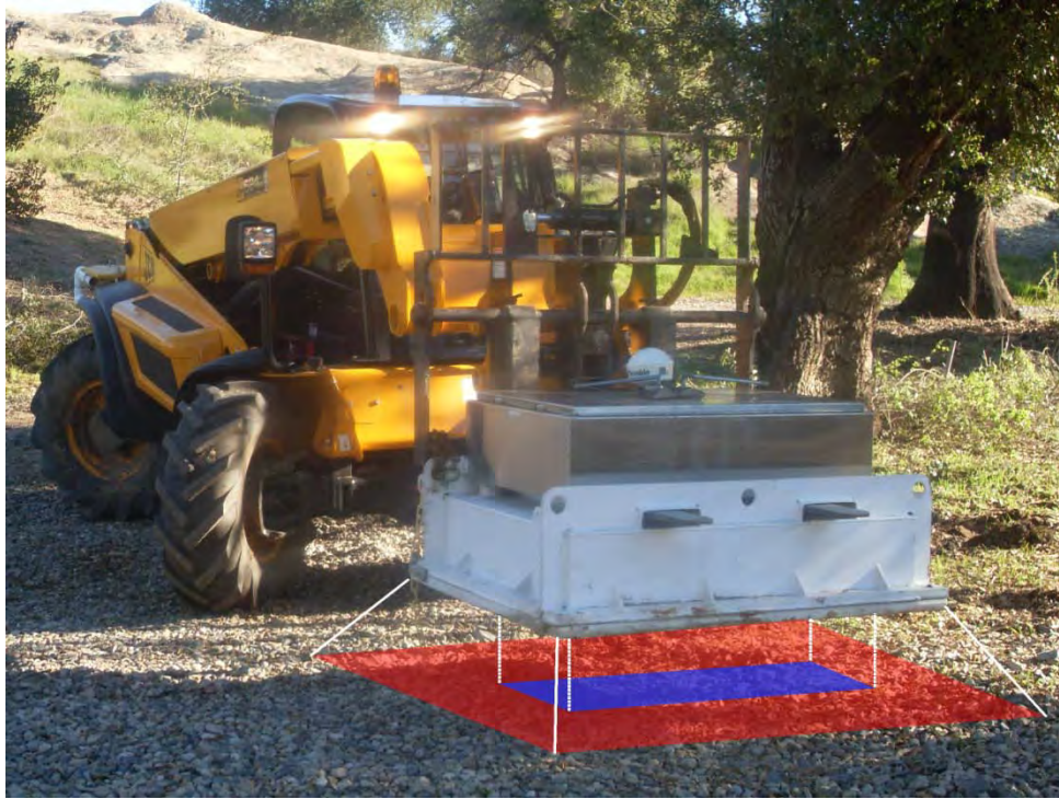
Figure 50 Illustration of Enhanced Radiation Ground Scanner II Field of View (Detector footprint in blue and FOV in red.)
