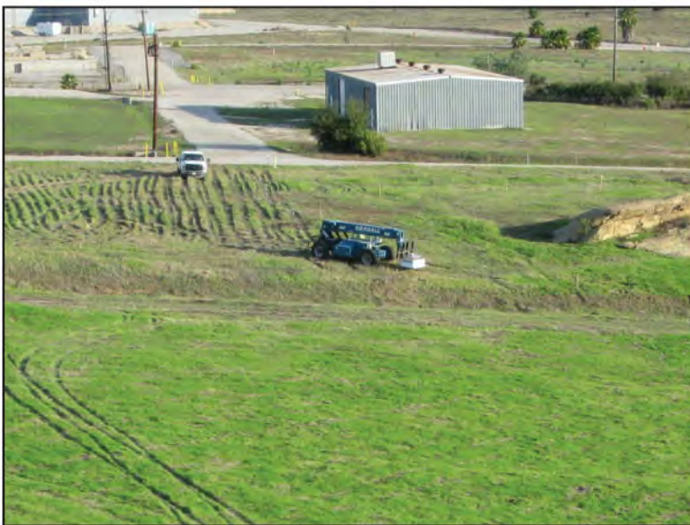
Plate 2A – ERGS vehicle conducting gamma scanning in SS-56 (Subarea 5D).
