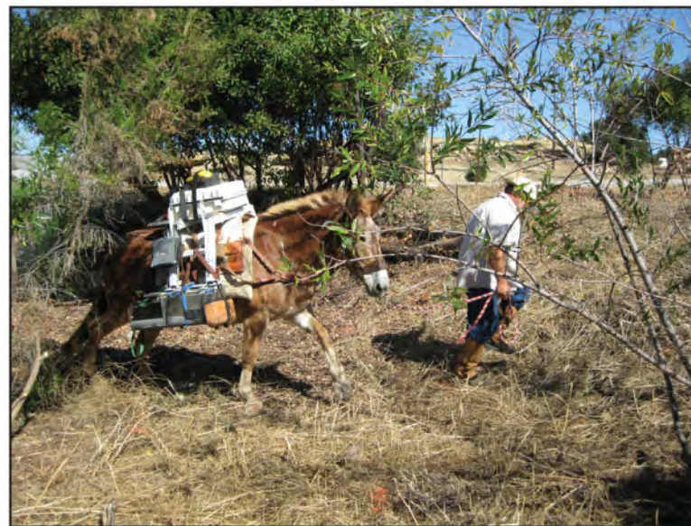
Plate 2B – Gamma scanning with mule-mounted scanner in SS-12 (Subarea 5B).
