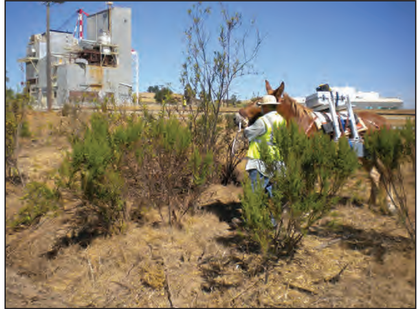
Plate 5B – Gamma Scanning activity via mule in SS-1.
