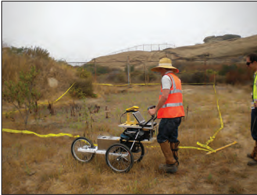
Plate 2A – Handcart scanner operator conducting Gamma Scanning in SS-8.
