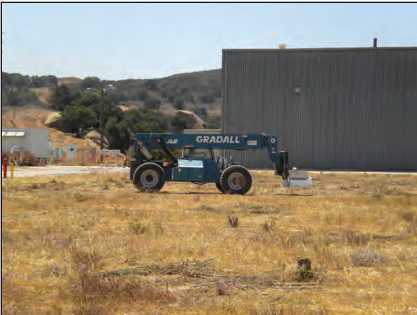
Plate 1C – ERGS vehicle conducting Gamma Scanning in SS-9.
