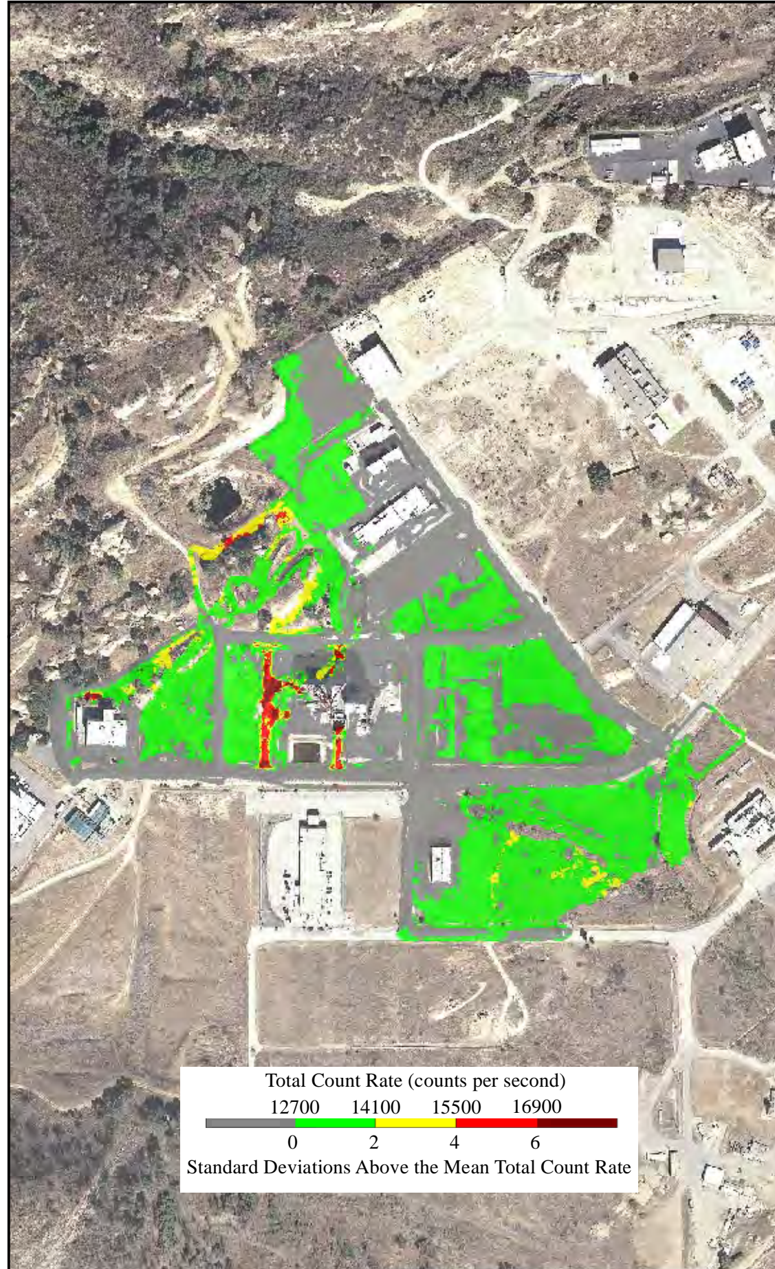
Figure 9.1 Comparison of Subarea 5C Scanning Results with Lang Ranch and Subarea 5C Backgrounds Santa Susana Field Laboratory
