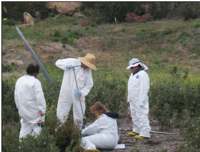
Photo 1C – Soil sampling with a hand auger in Subarea 6. Photo taken April 12, 2012.
