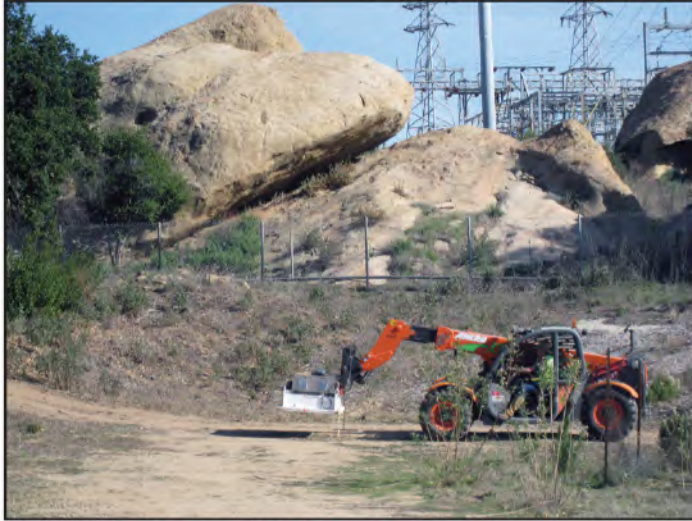
Plate 1A – Gamma scanning with the ERGS vehicle. January 10, 2012.
