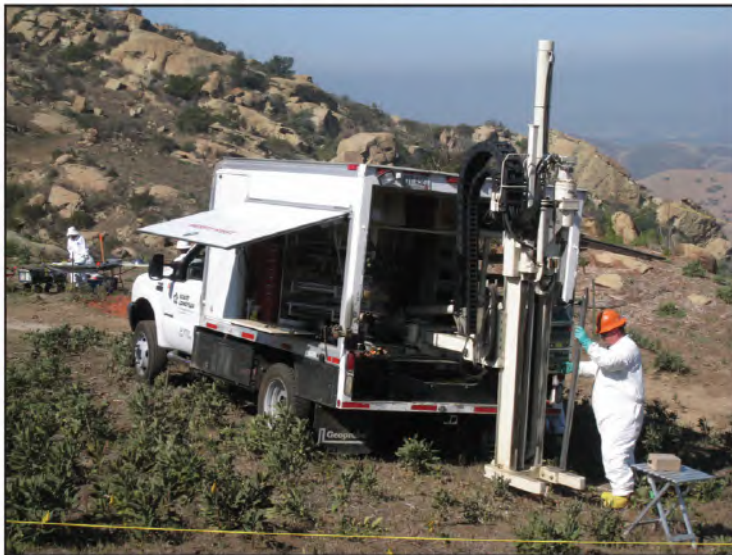
Plate 2C – Soil sampling activity using a Geoprobe DPT rig, in the NBZ. March 15, 2012.
