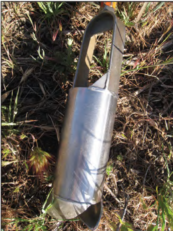
Plate 3C – Hand auger bit used for soil sampling activities during this quarter. March 20, 2012.
