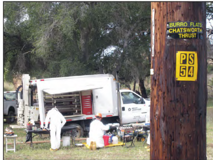
Plate 2D – Soil sampling activity using a Geoprobe DPT rig in Subarea 6. March 27, 2012.
