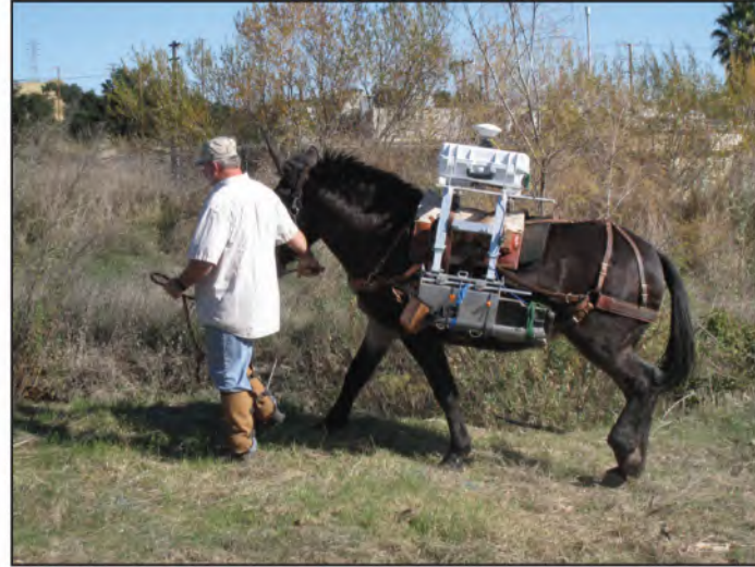
Plate 1B – Mule-mounted gamma scanning in Subarea 5C. January 5, 2012.
