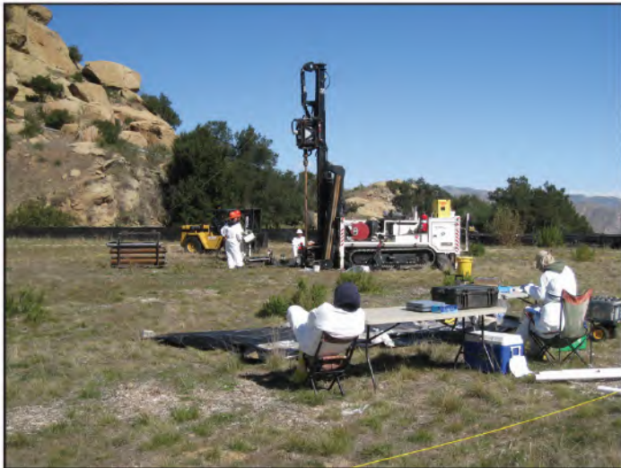
Plate 1C – Subsurface soil sampling activity in Subarea 6 using a drill rig. February 16, 2012.
