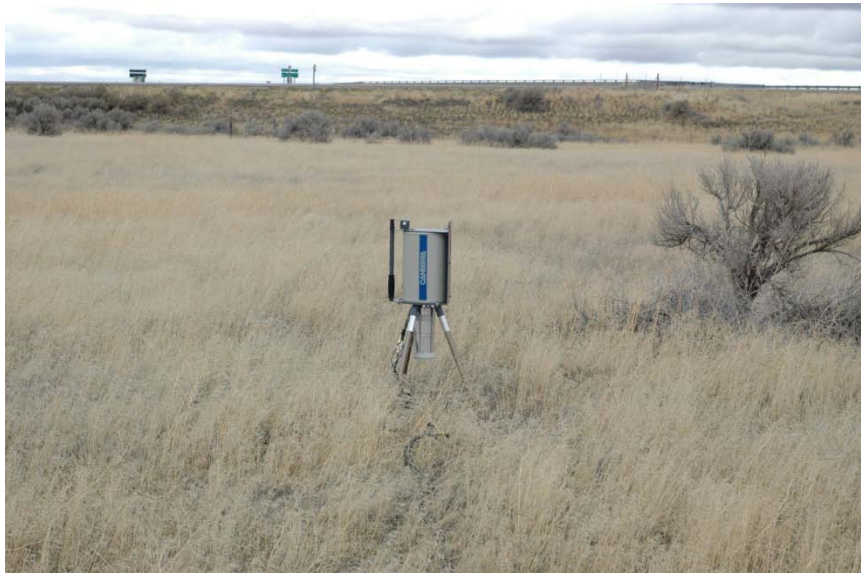
Photograph 6: HPGe Detector Mounted on a Detector Stand
