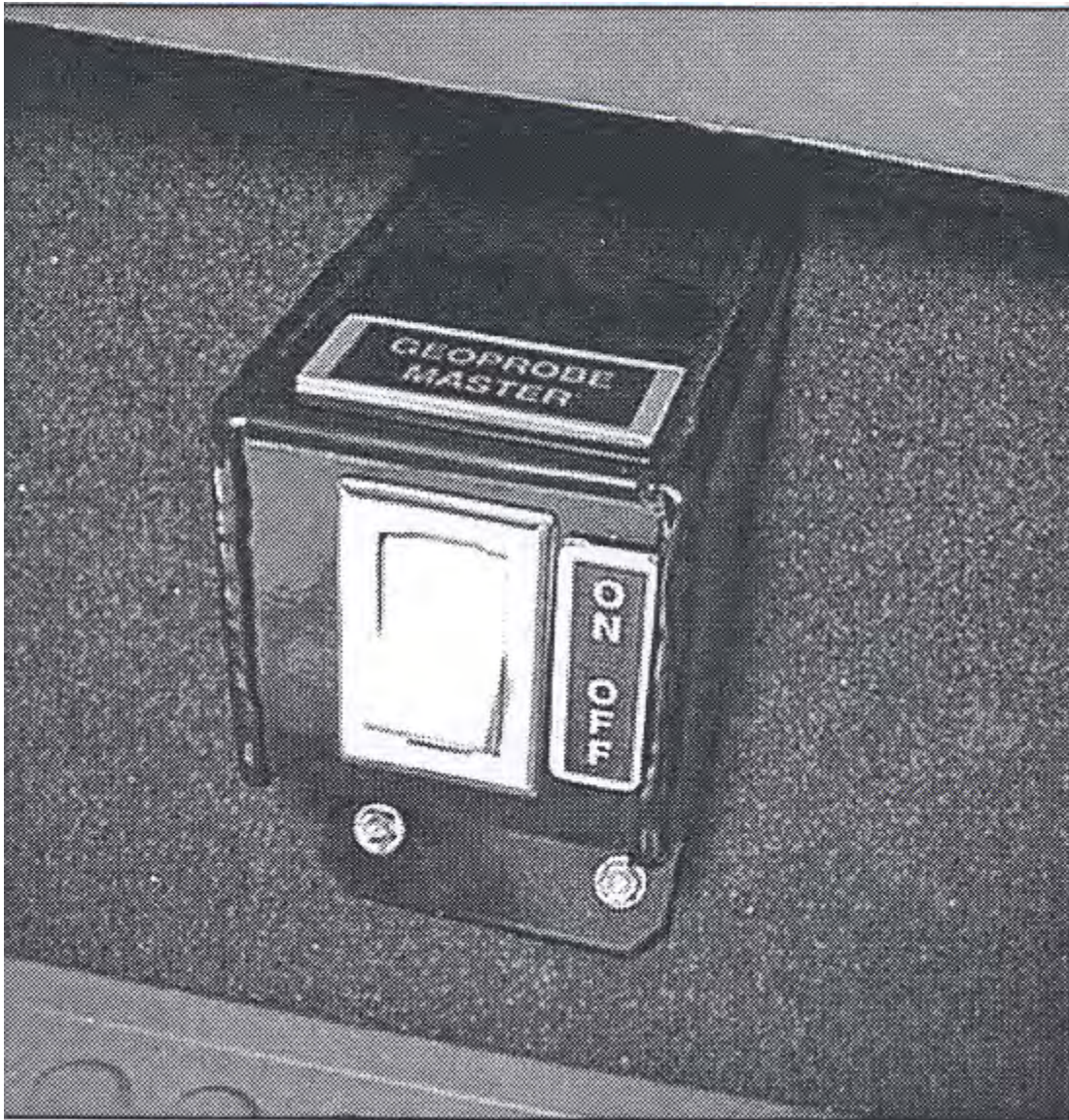
The Master Switch is mounted on the cab floor just inside of the driver-side door.
