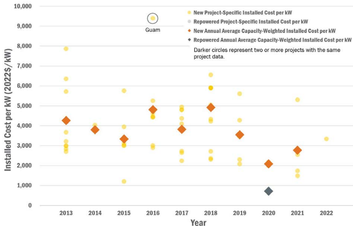
Figure 12. Annual average and project-specific new and repowered installed costs for projects using turbines greater than 100 kW, 2013–2022
