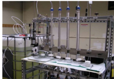
Packed columns to test removal of COCs from aqueous media
