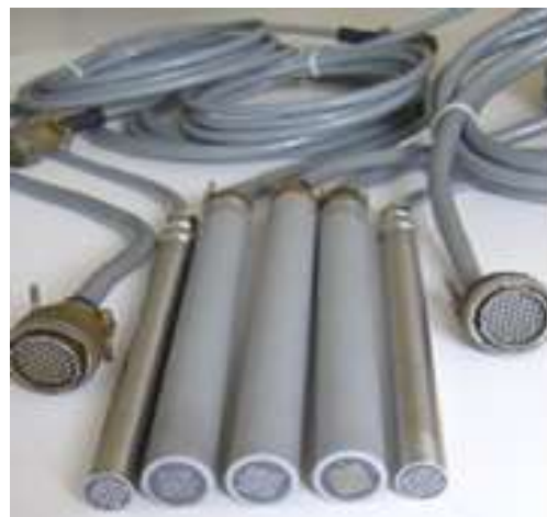
NanoCorr Tank Corrosion Probe
