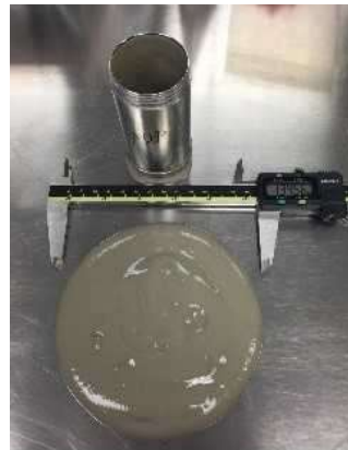
Grout Flow Testing of Encapsulation Grout
