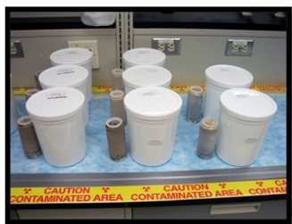
Grout Samples Curing
