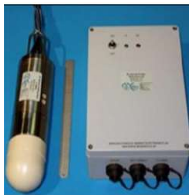
3D Profiling Sonar & Controller
