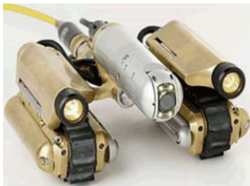
Versatrax 100 for Inspection of Small Pipe and Ducts
