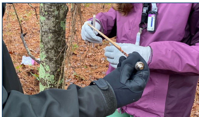
A core sample is extracted from a tree at the Savannah River Site (SRS). Tree ring samples were analyzed for total tritium content and tritium chemical speciation.
