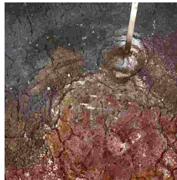
Sludge – Tank S-112
