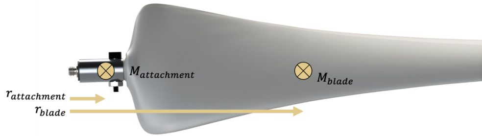
Figure 8: Centripetal Force Diagram
