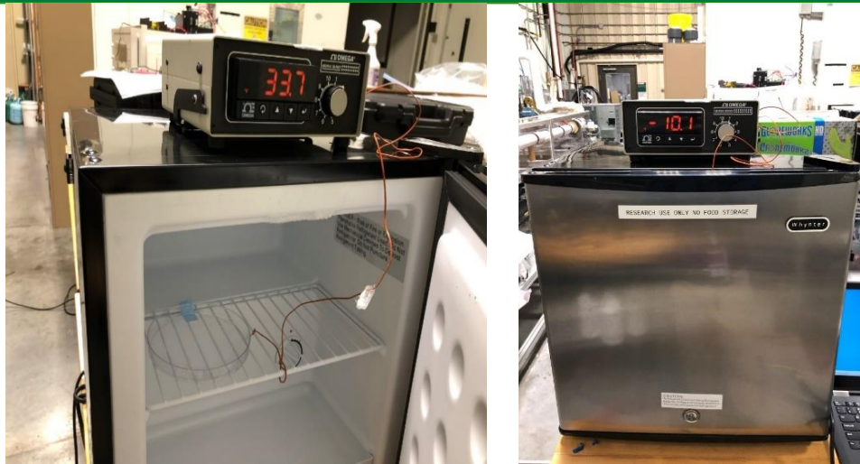
Test setup for cold-environment durability tests
