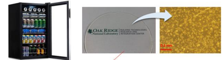
Enhanced: aerogel insulated glass unit
