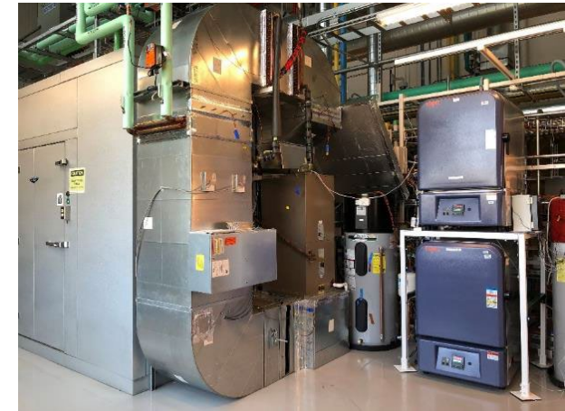
Environmental chambers for HVAC condenser and thermostat
