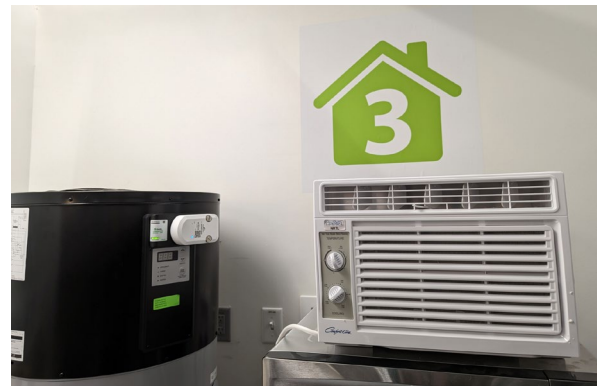
Heat pump water heater with communication module (left) and room air conditioners (right)
