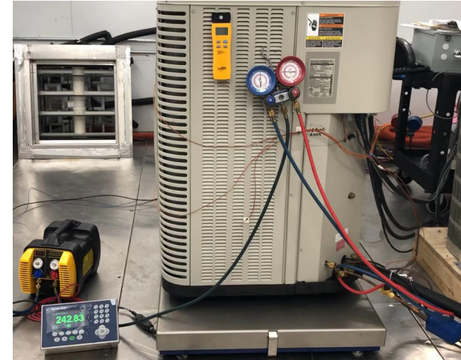
Outdoor unit of heat pump placed on a scale for charge migration measurement
