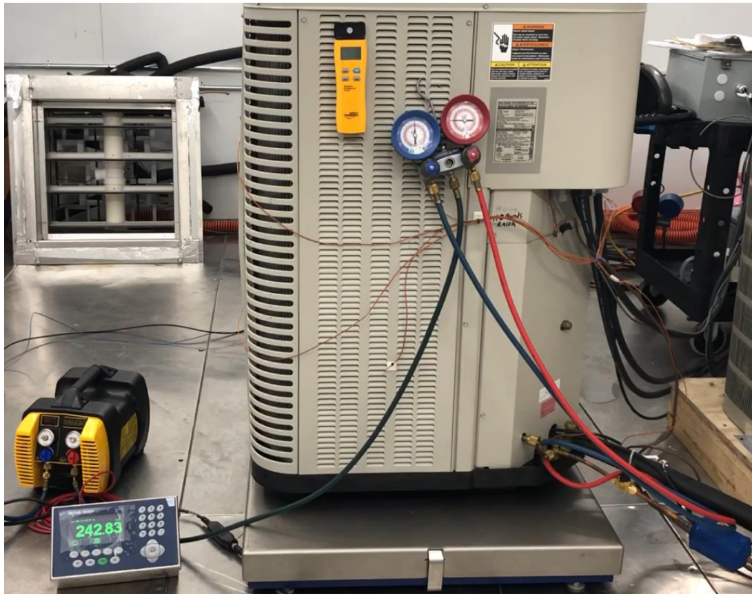
Outdoor unit placed on scale to measure refrigerant migration
