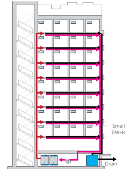
Hybrid HPWHs System With Sewer Heat Recovery
