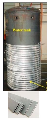
Working with Supplier to optimize microchannel geometry, balance between pressure drop and heat transfer @ target compressor size
