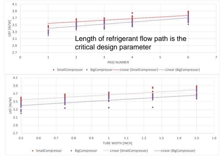
Extensive parametric study to identify optimized geometry
