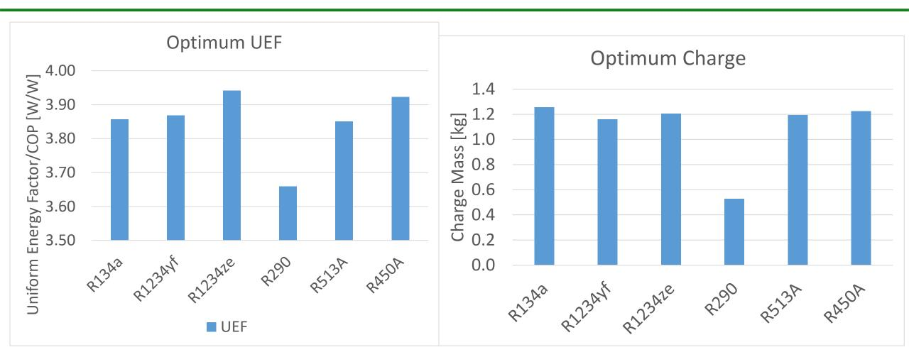
Propane HPWH can reach similar 24-hr heating efficiency (95%), and the required 50% charge of R-134a because of propane's small molecular weight.
