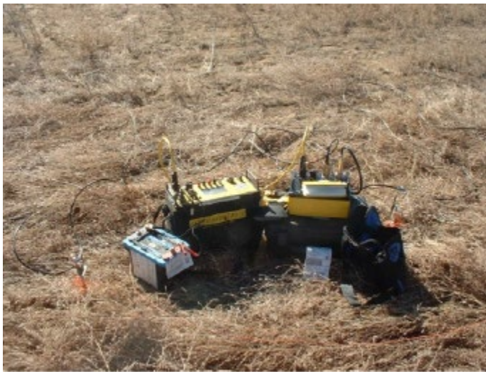
Figure 3. Resistivity system deployed in the field. Note the cables connected to the electrodes in the background, with the 12V battery, AGI SuperSting R8 Control unit, and a SwitchBox. A similar system will be deployed at the CFPP site except multiple switch boxes will be employed to handle the proposed electrode configuration.
