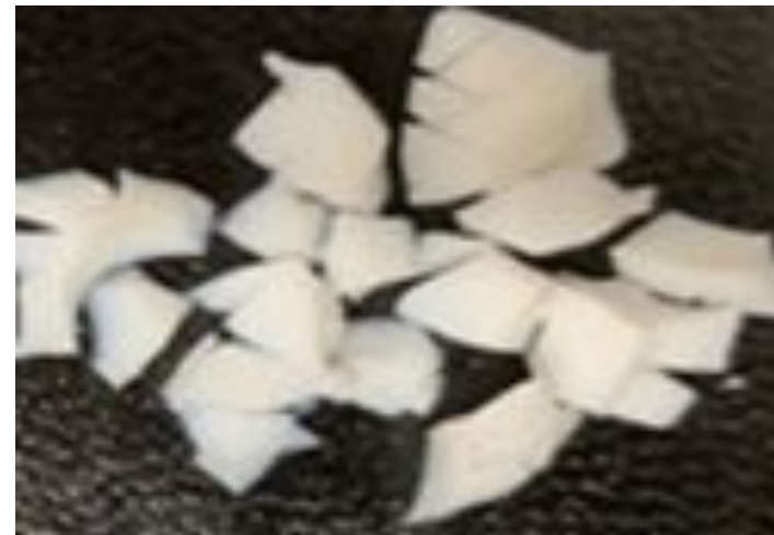
Aerogels reinforced with clay
