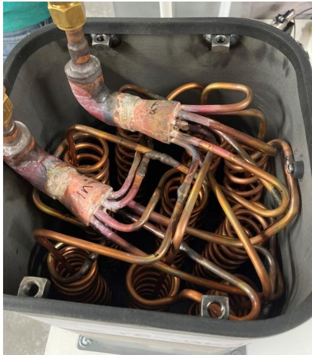
First Simple Heat Exchanger Prototype Built
