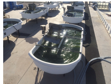
Standard 4.2 m 2 open raceway ponds (ORP) for SOT cultivation trials at AzCATI. Typically run simultaneously in triplicate.
