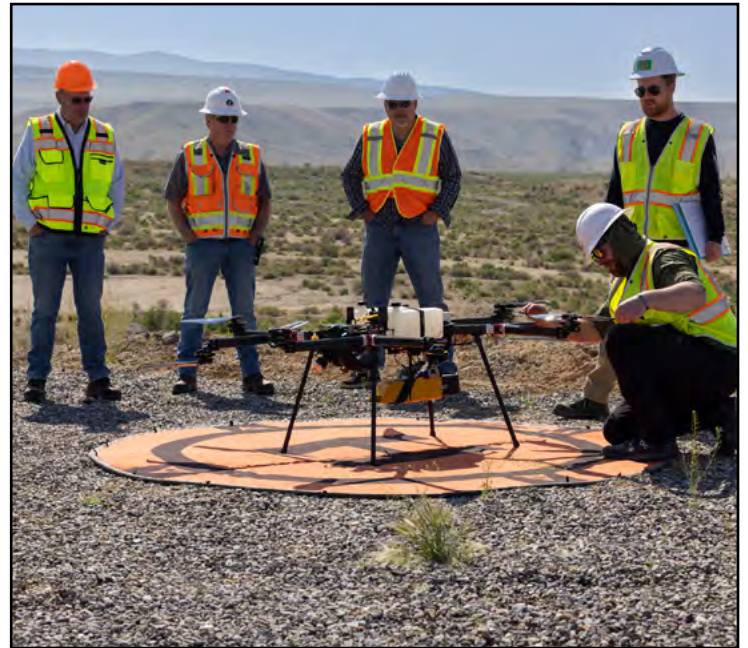
The aviation team and LM Support contractors watch drone-launch preparations for a baseline aerial survey at the Grand Junction site on May 23.
