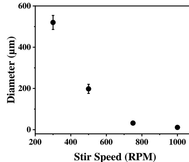
Demonstrated encapsulation of iso- and epoxy-based reactive agents with tunable diameters
