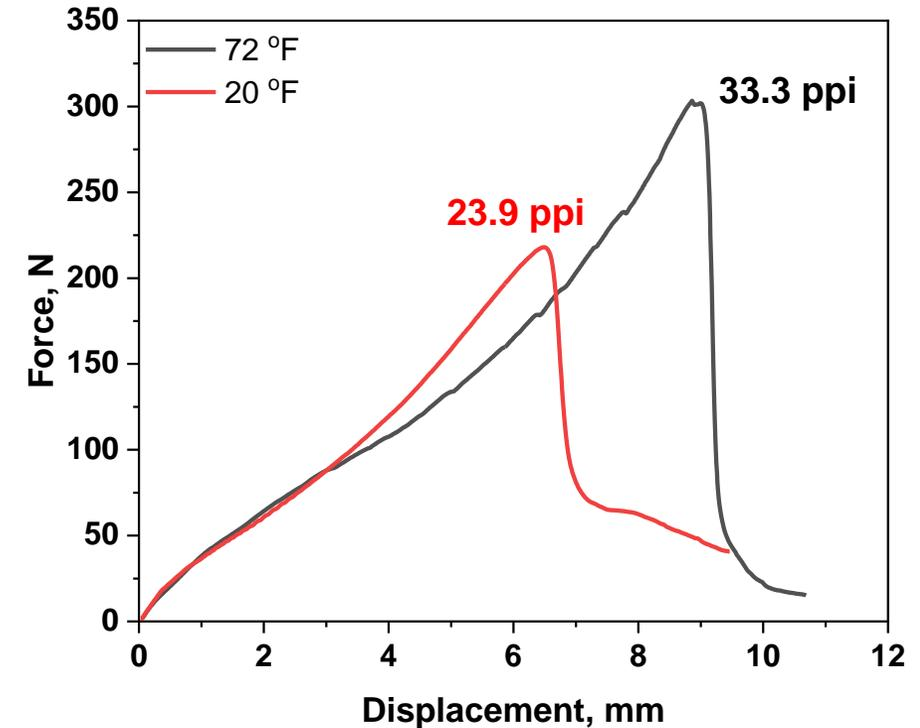
Nonoptimized epoxy-based formulation exceeded 20 ppi peel strength target after curing at ambient and 20°F for 21 days
