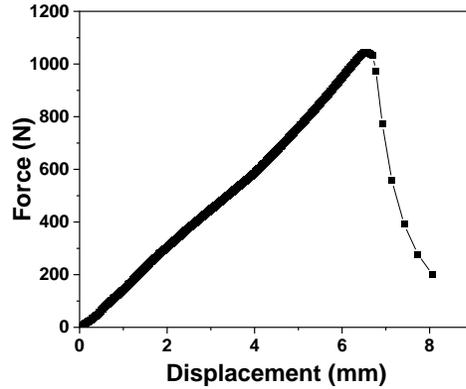
119 ppi peel strength after 75 psi trigger and 3-day curing
